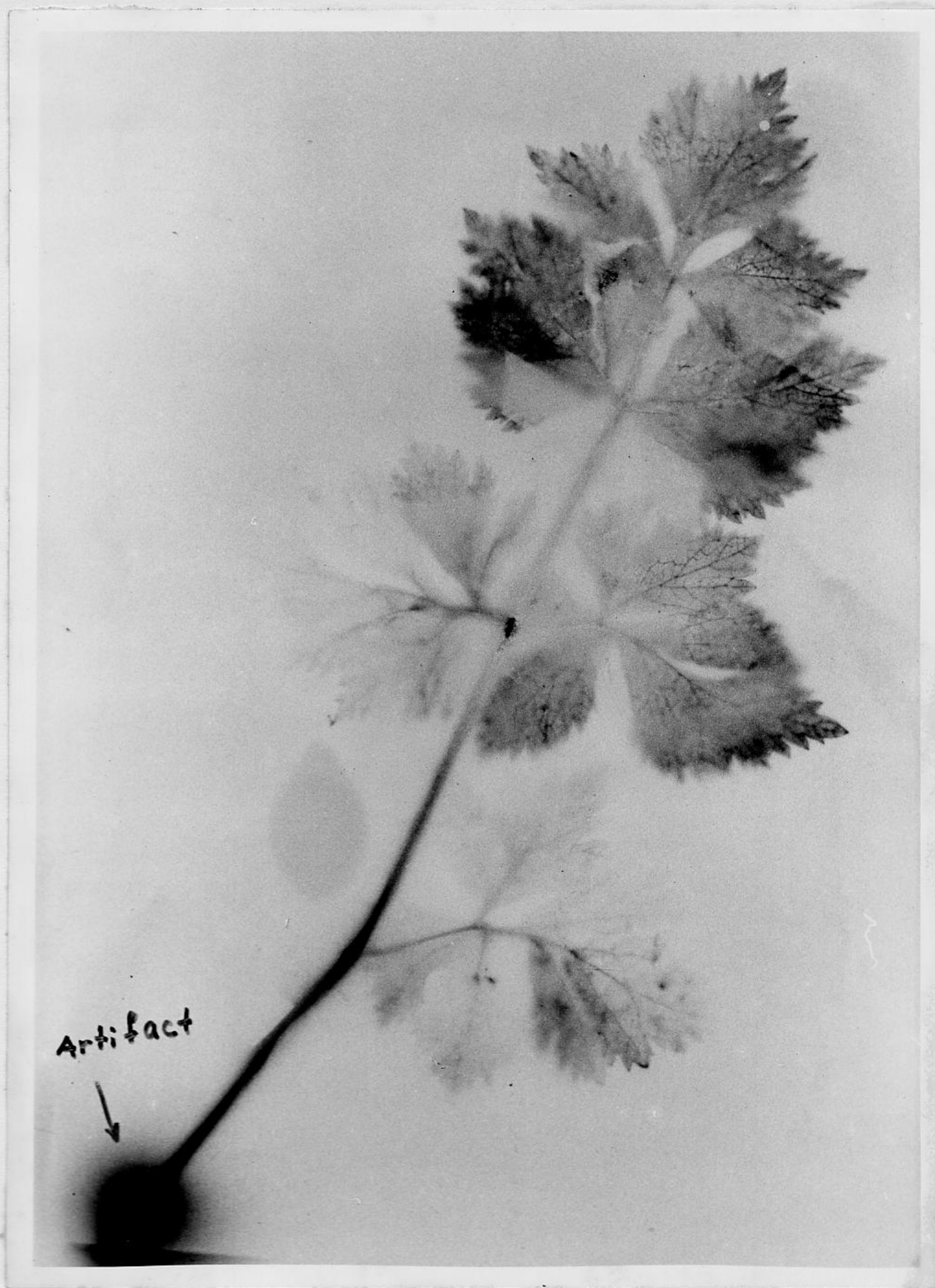
Figure 3. Autoradiograph of a celery shoot which was injected with iron-59 and was processed without freezing (10-day exposure to film).
