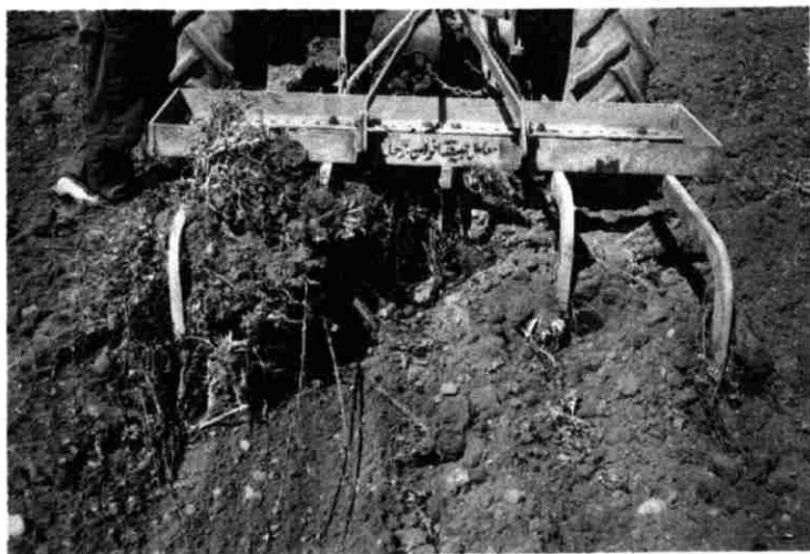
Figure 23. Intercultivation of orchard with the new design.
