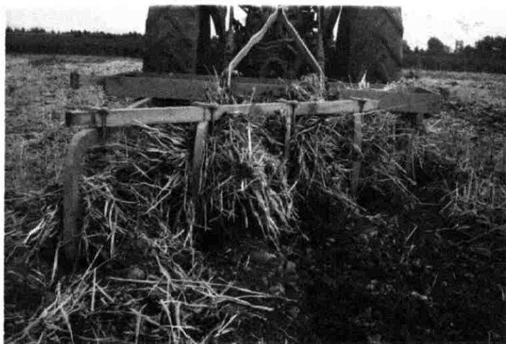
Figure 22. Old design plowing a field with wheat stubble mulch.
