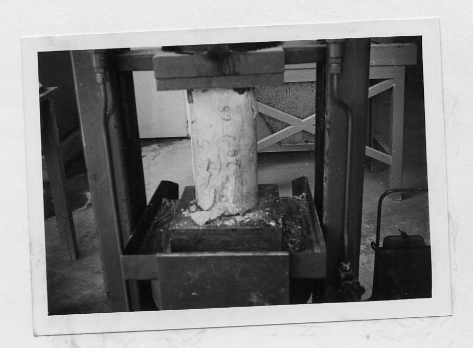
Figure 6. View of the Vertical Cracks Developed in a Concrete Cylinder Subjected to Unconfined Compressive Test.
