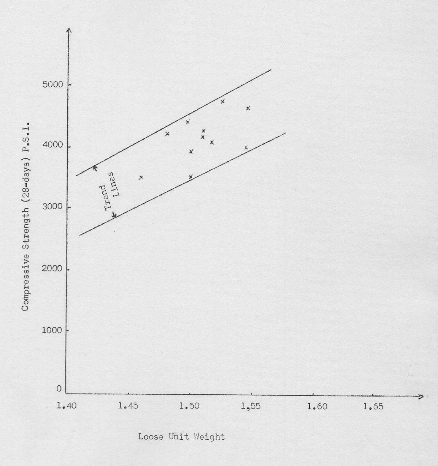
Figure 8. Relationship Between Compressive Strength (28-days) and Loose Unit Weight.
