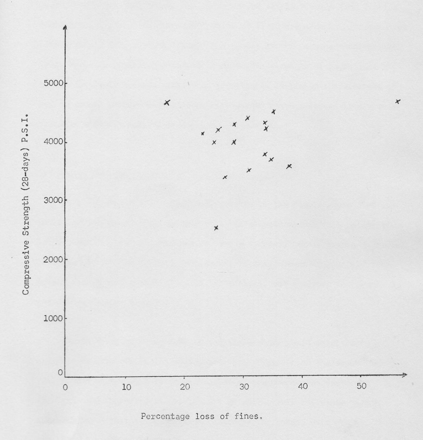
Figure 7. Compressive Strength (28-days) Versus Percentage
