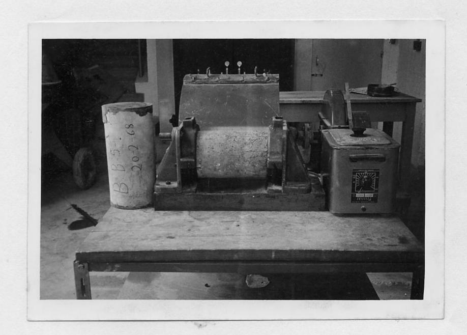
Figure 4. Soiltest Apparatus Used for Capping Cylindrical Concrete Samples.
