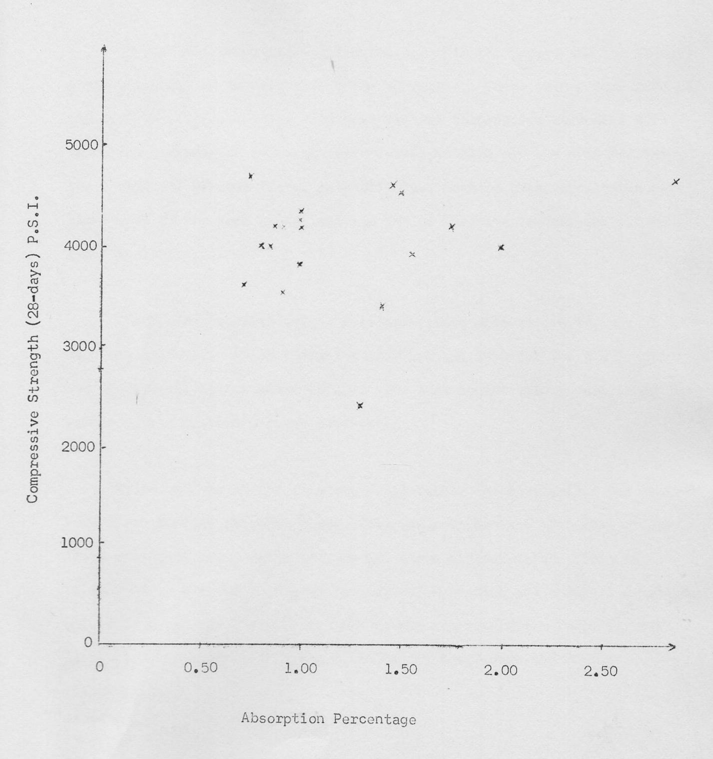
Figure 11. Relationship Between Compressive Strength (28-days) and Absorption Capacity.
