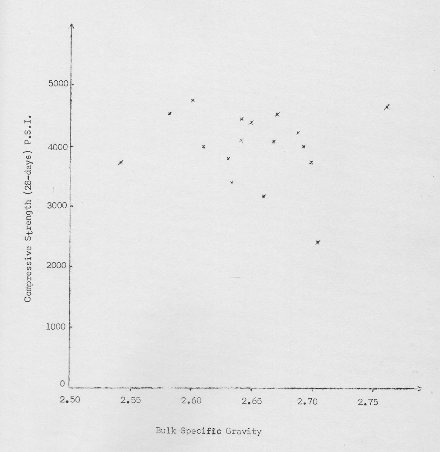
Figure 10. Relationship Between Compressive Strength (28-days) and Bulk Specific Gravity.
