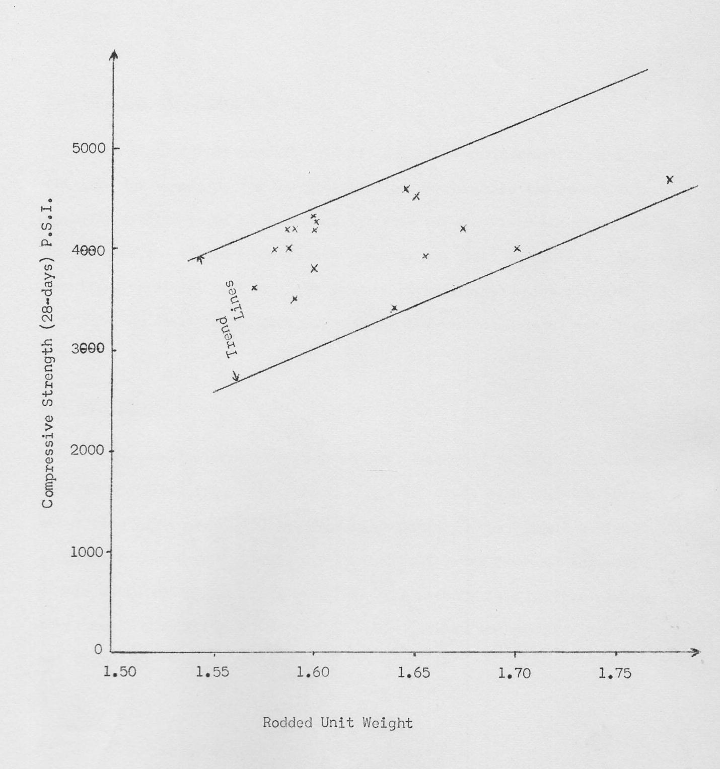
Figure 9. Relationship Between Compressive Strength (28-days) and Rodded Unit Weight.
