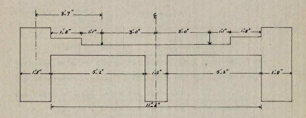
With the loads so placed, the center beam sustains  $\frac{3.58 \times 2}{6.333}$  = 1.13 times the value of each wheel load. Therefore 10,000 x 1.13 = 11300 lbs from the rear
