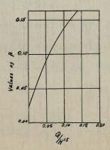
After Computing the value of  $\frac{Q}{H1.5}$  which  $\frac{5.2}{27 \ 1.5} = 0.037$  a value of B = 0.075 is taken from this chart, and the correct heiht of the sill for satisfactory energy dissipation is then BH = 0.075 x 27 = 2m.
