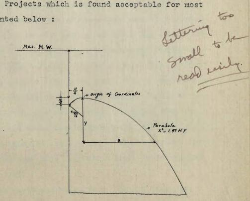
The curve on the downstream side is defined by a parabola which can be approximated by a compound curve of two radii for simplified construction.
