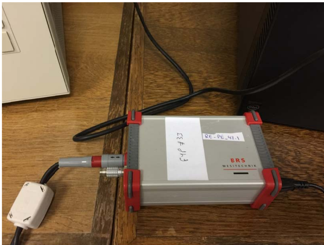
Figure 17. The BRS device used for electro-impedance spectrometry
