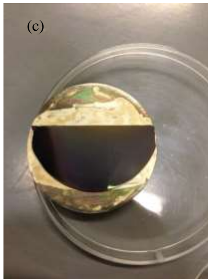
Silicon pieces glued on the metal plate for samples (a) I, (b) II and (c) III
