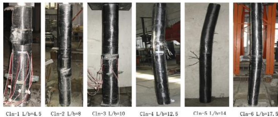
Figure 4. Columns with different slenderness ratios, Placet et al.
