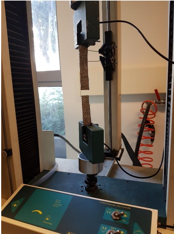
Figure 21. Tensile test setup for hemp fabrics.
