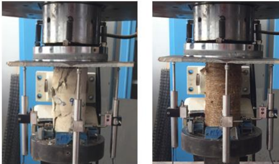
Figure 11. Preliminary study: Uniaxial compression test setup.
