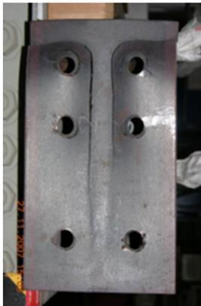
Fig. 6. Time-independent endplate deformation of flush endplate connections at 450°C
