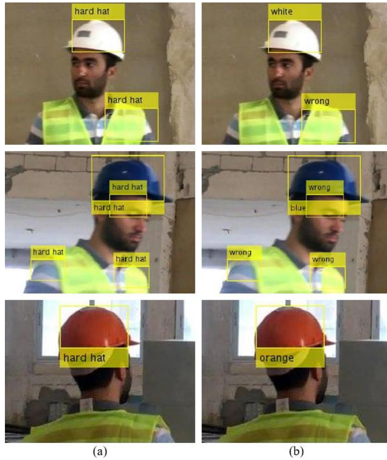
Figure 3.31: Hardhat detection results for positive images, (a) Cascade object detector, and (b) Cascade object detector and color segmentation
