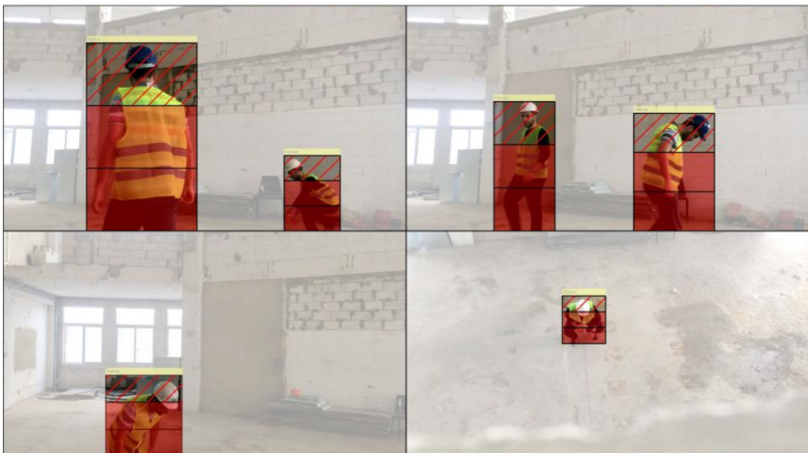
Figure 3.28: Hardhats worn by workers – Inside the region of interest
