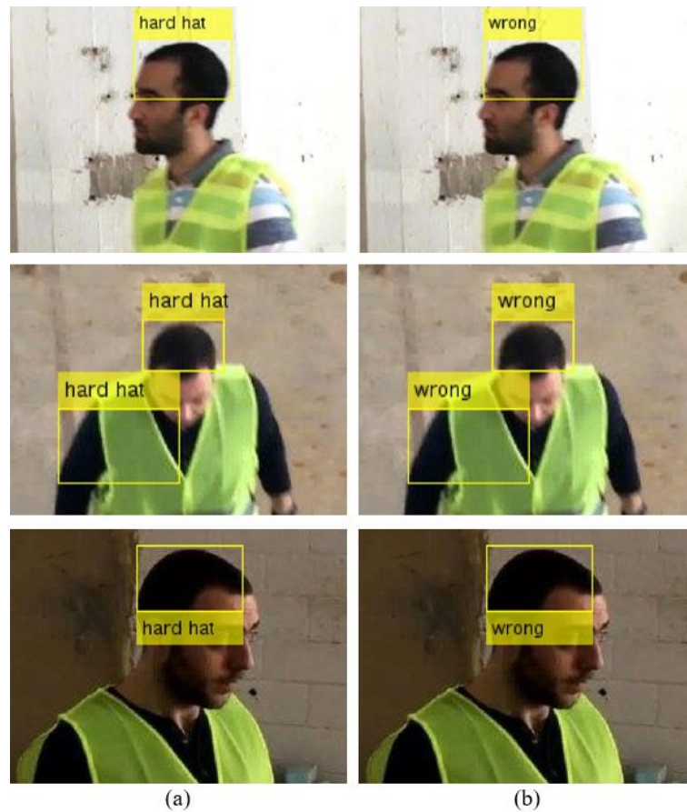
Figure 3.32: Hardhat detection results for negative images, (a) Cascade object detector, and (b) Cascade object detector and color segmentation
