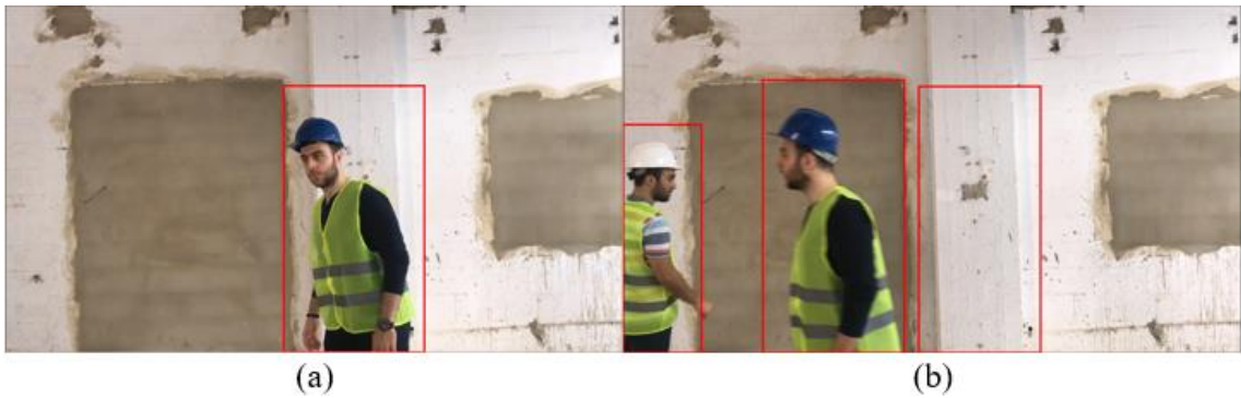
Figure 3.24: Background Subtraction: (a) Initial detection, and (b) Wrong detection in initially detected region
