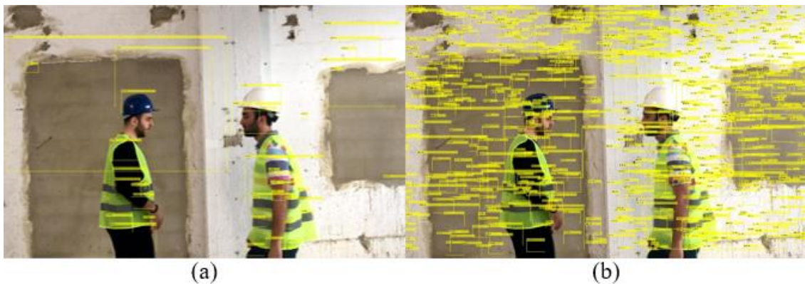
Figure 2.9: High rate of incorrect detections: (a) Using Haar Features, and (b) Using LBP Features
