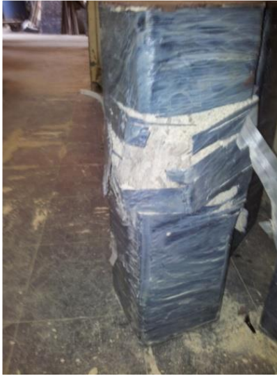
Figure II-3 - Typical failure modes of specimens: (a) Confined – (b) Unconfined
