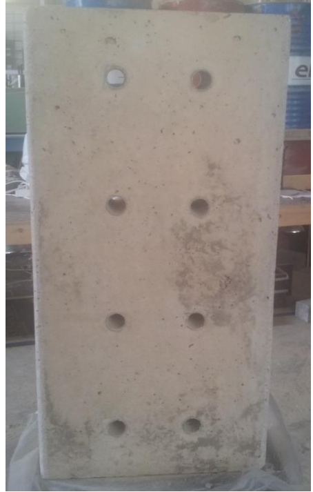
Figure AI- 3 – Cured concrete specimens after removal of PVC pipes
