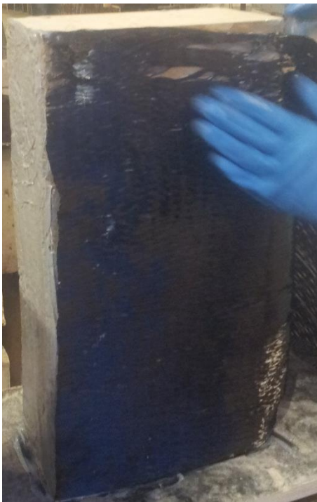
Figure AI- 4 – Wrapping and adding anchors to cured concrete specimens
