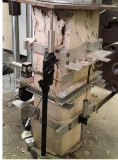
Figure II-3 - Typical failure modes of specimens: (a) Confined – (b) Unconfined
