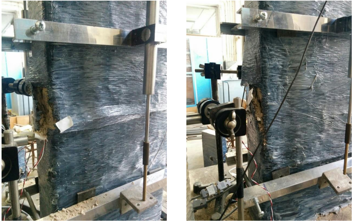
Figure AI- 5 – Typical failure of anchored specimens
