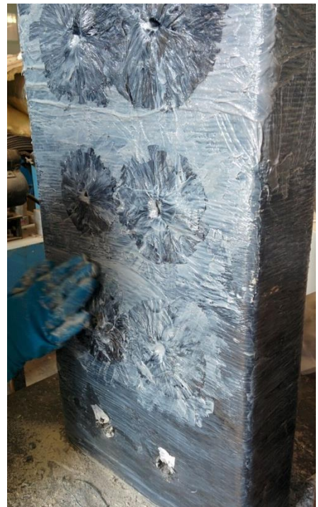
Figure AI- 4 – Wrapping and adding anchors to cured concrete specimens
