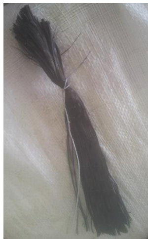
Figure I-2 - FRP anchor prepared by folding a strip of the FRP sheet
