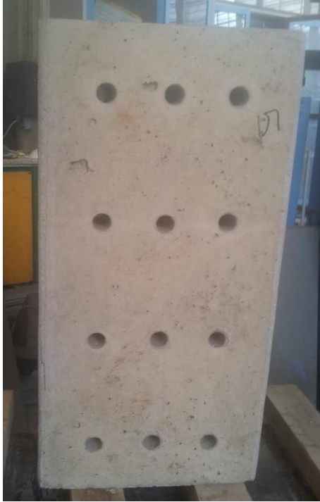
Figure AI- 3 – Cured concrete specimens after removal of PVC pipes
