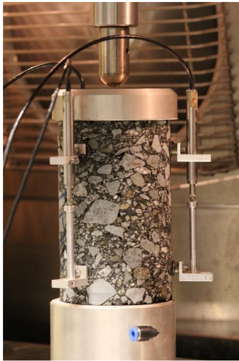
Figure 11. Complex modulus testing setup.
