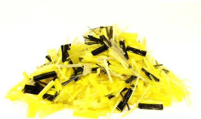
Figure 7. Mix of aramid and polyolefin fibers.
