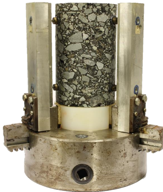
Figure 10. Gluing jig for mounting studs on asphalt samples.
