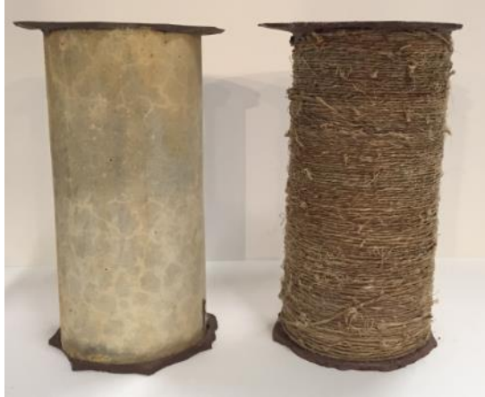
Figure 3.4 Control (Left) and Hemp-Confined (Right) Specimens.
