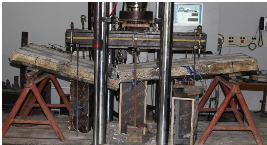
Figure 4.18 Failure Mode of H1-a.
