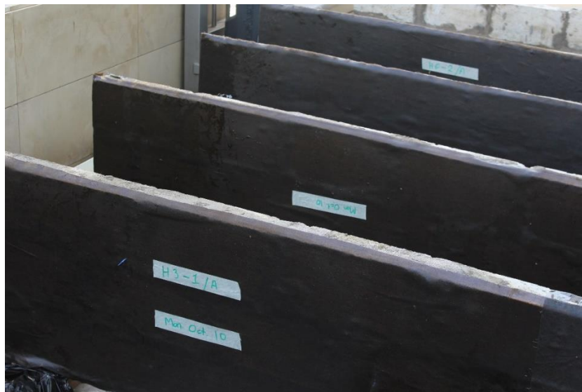
Figure 3.15 Strengthened Test Wall Specimens.
