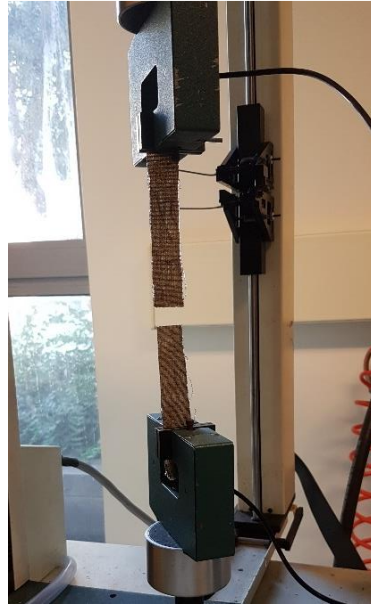
Figure 3.9 Tensile Test Setup of Hemp Fabrics
