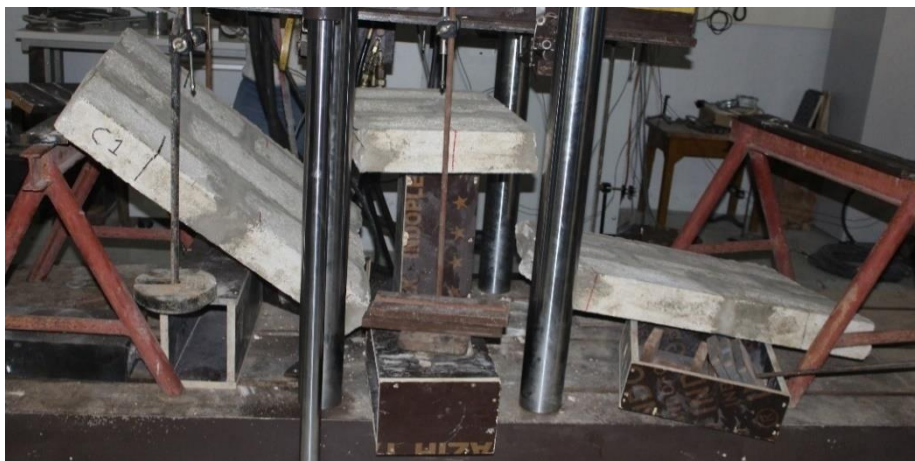
Figure 4.17 Failure Mode of Control Wall C1.
