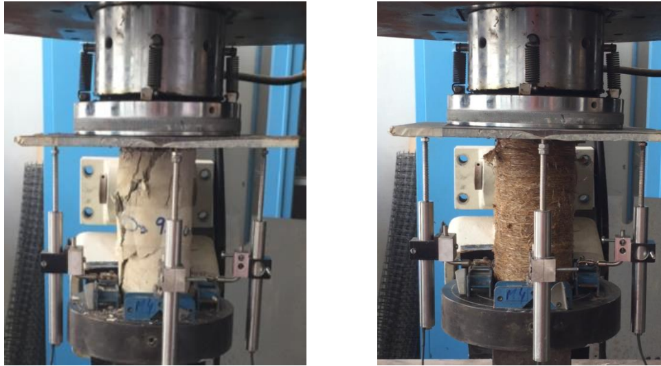
Figure 3.5 Test Setup for Compression Test of a Control Specimen (Left), and a Hemp Specimen (Right).
