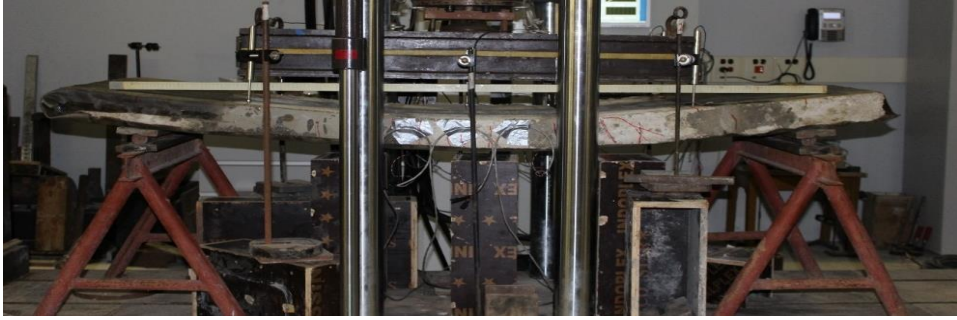
Figure 4.28 Deflected Shape of Wall H3-b.
