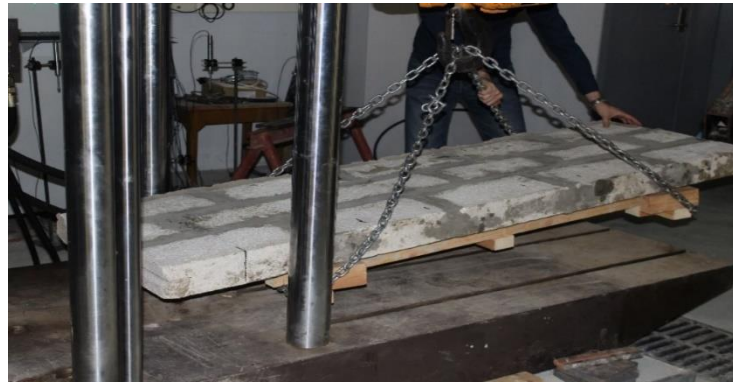
Figure 3.30 Positioning Wall Specimen into MTS Machine.
