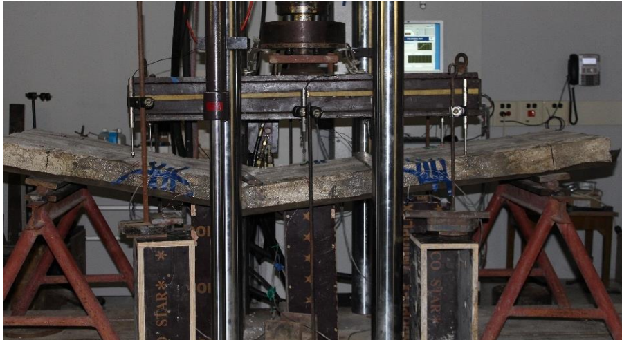
Figure 4.20 Failure Mode of H1-b.
