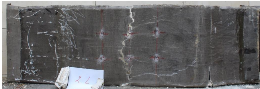
Figure 4.27 Failure Mode of H3-b.
