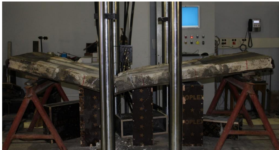
Figure 4.24 Failure Mode of H2-b.
