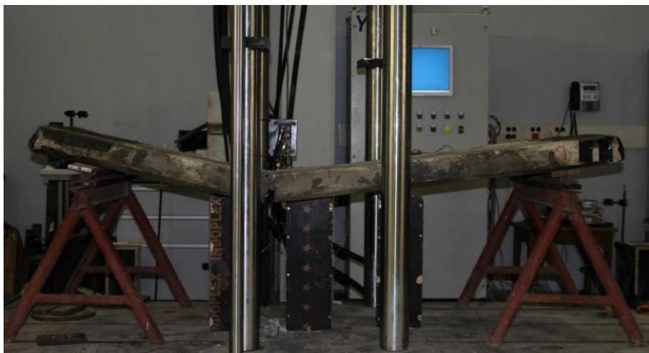
Figure 4.22 Failure Mode of H2-a.
