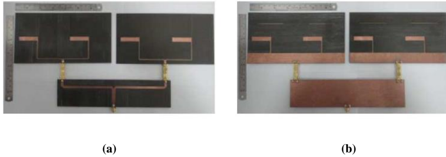
Figure 7: Photographs of the 1by4 quasi-Yagi array: (a) Top side, (b) Back side. [16]
