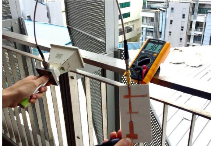
Figure 12: Measurement of harvested DC voltage from ambient. [23]
