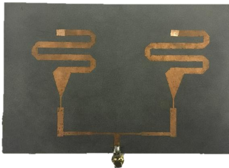
Figure 43: Photo of fabricated meander antenna array.
