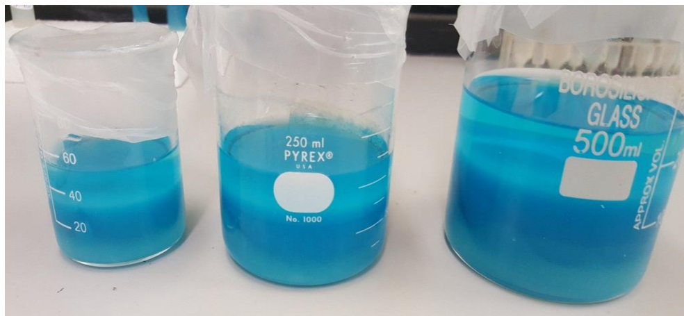
Figure 2. 7. MOF-199 prepared via RDF process at different scales
