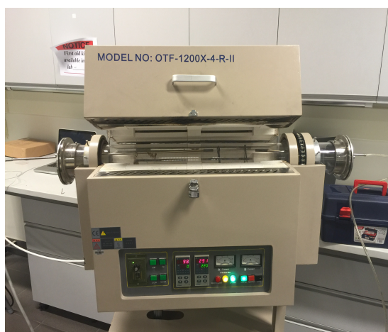
Figure 13 Electric furnace unit
