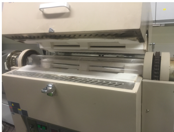
Figure 14 Thermal furnace heating compartments
