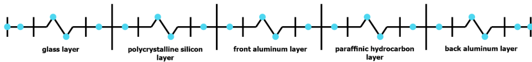
Figure 3.6: Outdoor PV/PCM module 1-D model
