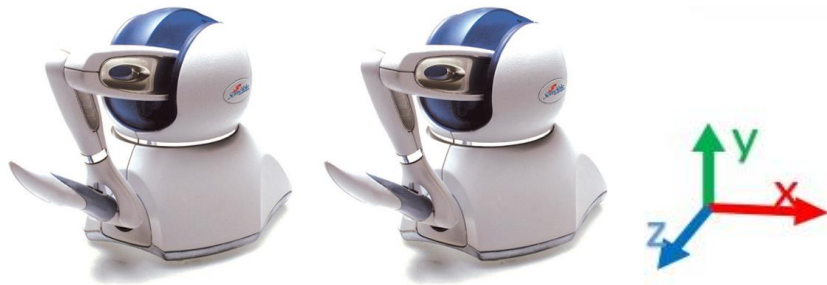
Figure 3: Haptic joysticks with the UAV axis
