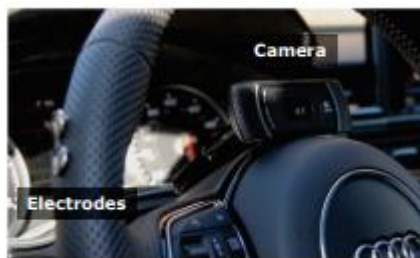
Figure 35: Camera installed on the steering wheel to measure heart rate (Hernandez et al., 2014)
