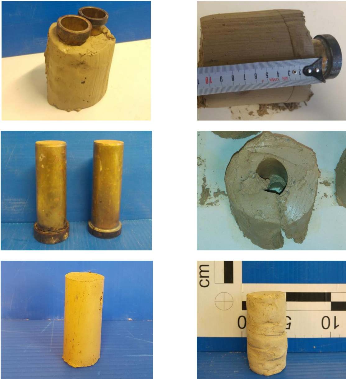
Figure 10. UU test Sample
