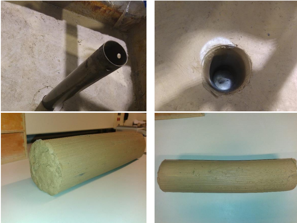
Figure 8. The procedure of installing a Shelby tube
