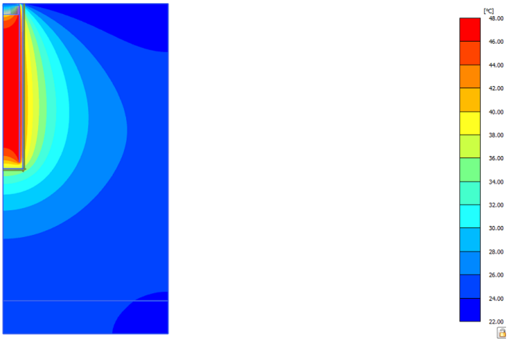
Figure 57. Temperature variation in soil at the end of heating phase in Plaxis 2D
