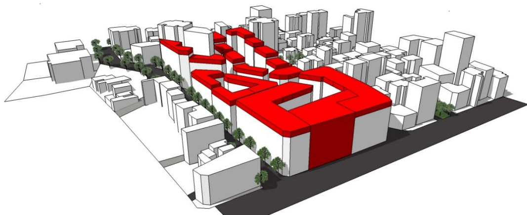
Figure 114: North-East Axonometric of Al-Tamlis Revised. In red, the increase in density and enlargement of the Frontage of the Mixed-Use Center
