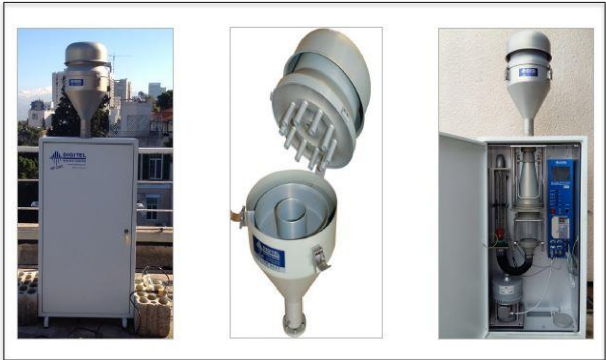
Figure 9. From left to right: the high-volume sampler, the PM 10 sampler impactor, and the HVS compartments constituting it
