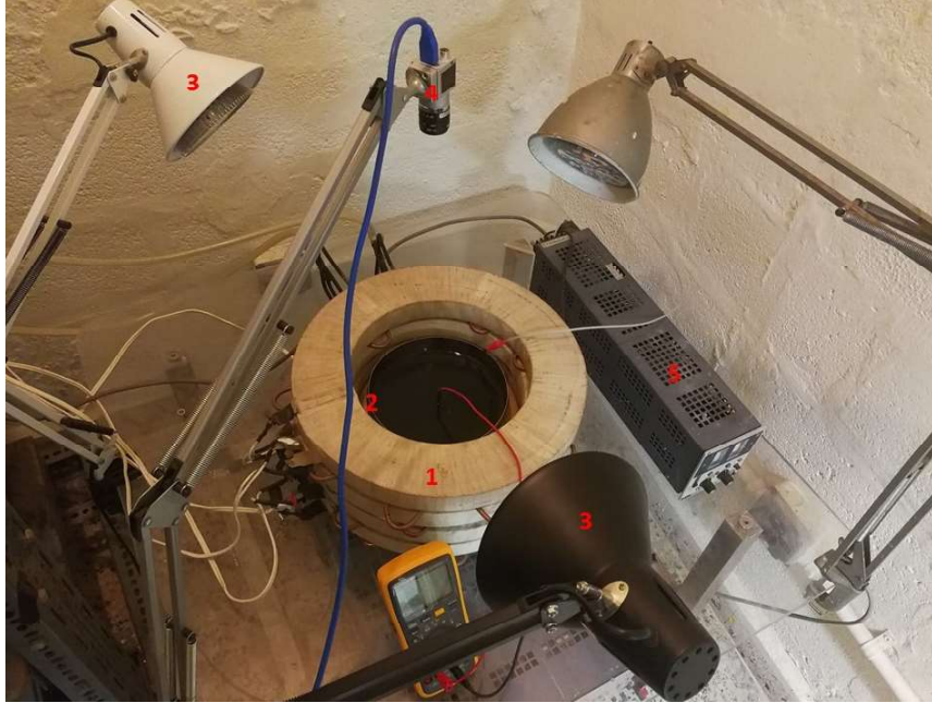
Figure 2.1: This figure shows the experimental setup used. (1) indicates the electromagnets, (2), the cylinder with the inner and outer electrodes, (3), the UV lights, (4) the camera and (5) the power supply used to pass the current in the fluid.
