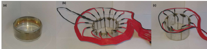
Figure 3.11: (a) container with outer one continuous sheet electrode. (b) container with 16 outer electrodes. (c) container with 8 outer electrodes. All with a radius of 4.6 cm.
