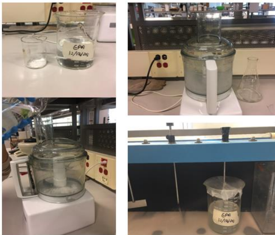
Figure 18: Preparation of xanthan gum fluids
