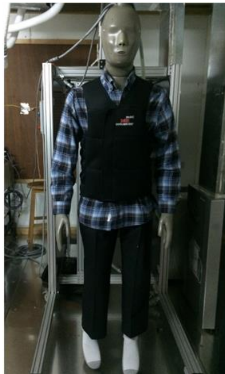
Fig. 9: Picture showing Newton thermal manikin clothed with the PCM cooling vest
