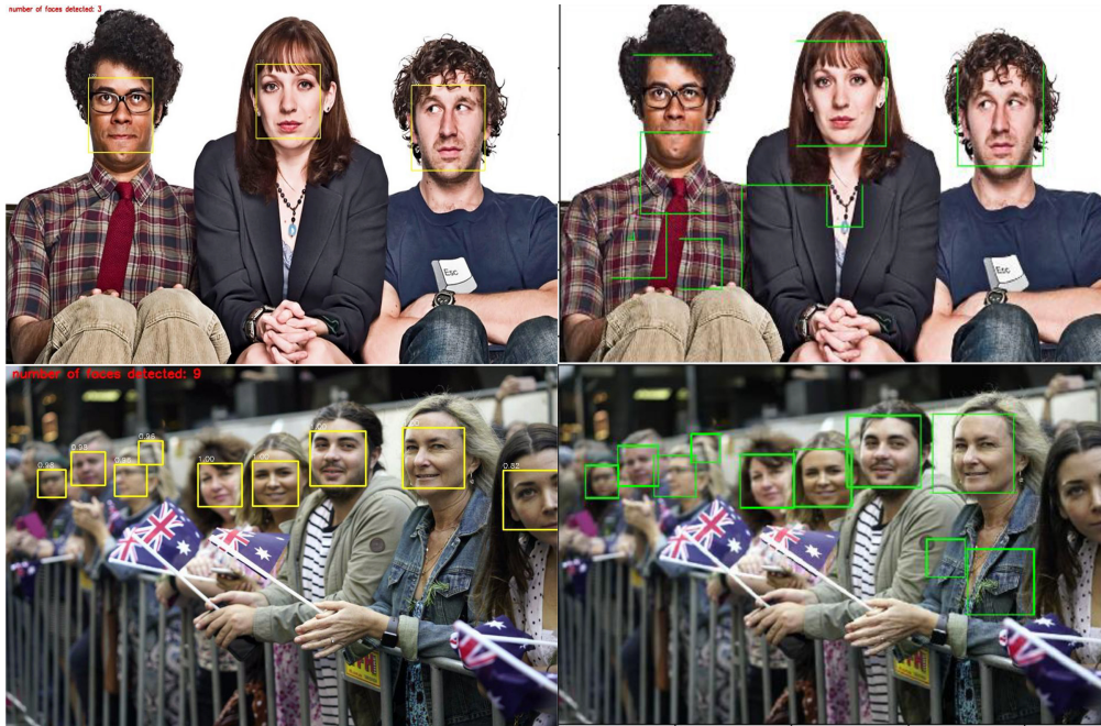
Figure 3.2: Results showing YOLO face detection to the left Haar Cascade face detection to the right
