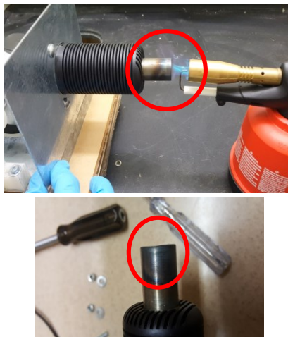
Figure 77. Hot zone on the Expansions Cylinder
