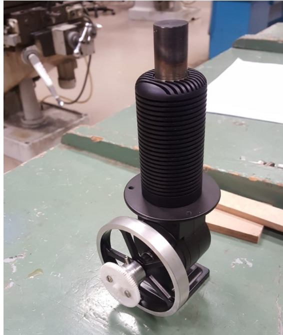
Figure 75. Beta-Stirling Engine from GreenPowerScience with adaptor and gear addition
