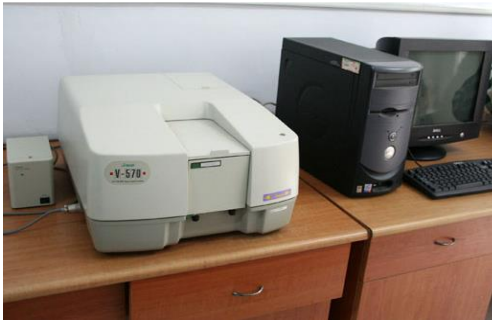
Figure 3.4. The V570 Model UV-VIS Spectroscopy Used.
