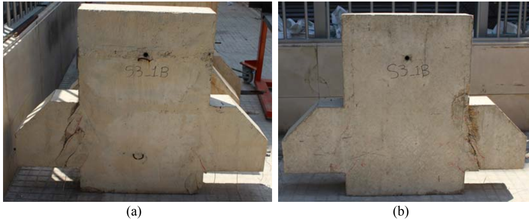
Fig. 12: Specimen S3-1B after failure: (a) Front face, (b) Back face
