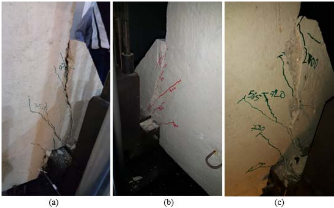
Fig. 9. Failure pattern in specimens: (a) C1-0B, (b) S1-1B, (c) S1-2B.
