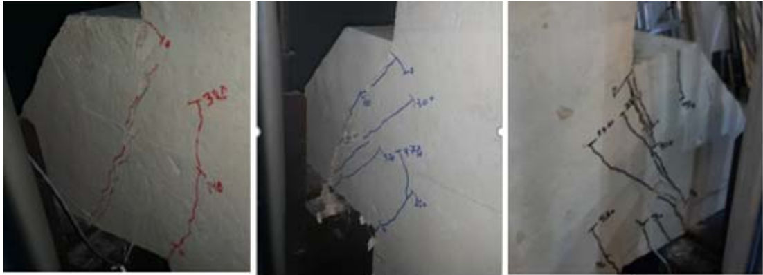
(a) (b) (c) Fig. 10. Failure pattern in specimens: (a) C2-0B, (b) S2-1B, (c) S2-2B.
