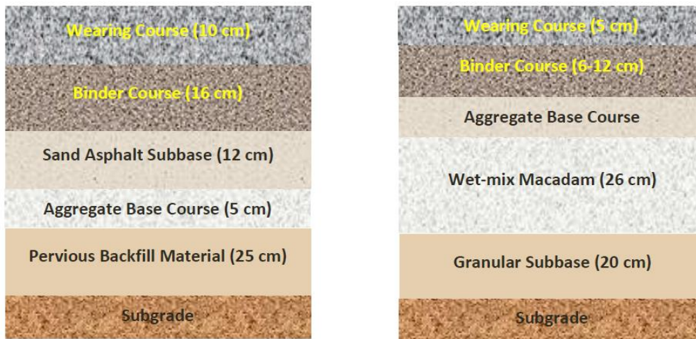
Figure 4.7: Typical Pavement Cross-Section for roads in Abu Dhabi (left) and roads in Dubai (right) (Chehab, 2016)
