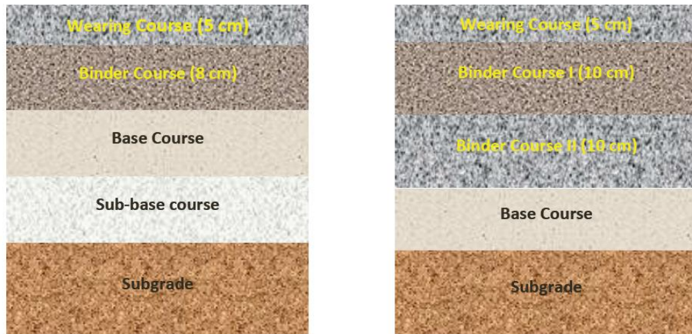
Figure 4.6: Typical Cross Section of Roads KSA (low, high) (Chehab, 2016)
