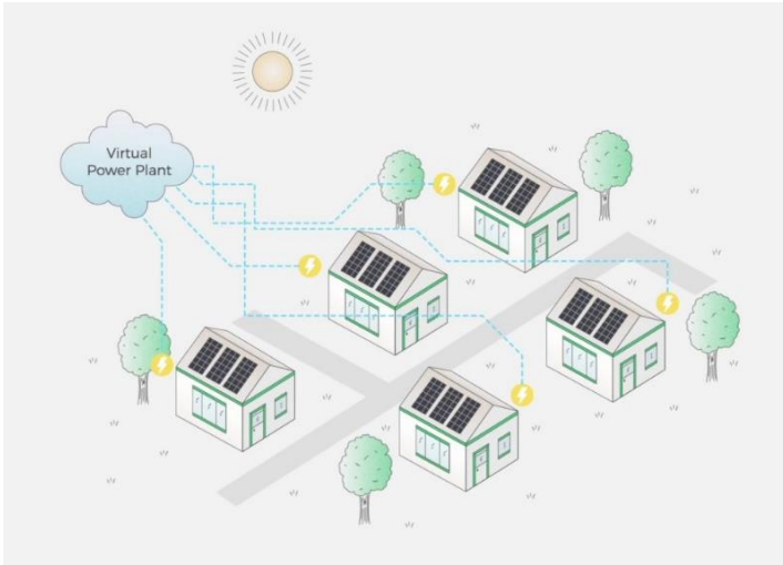
Fig 31: Virtual PV power plant
