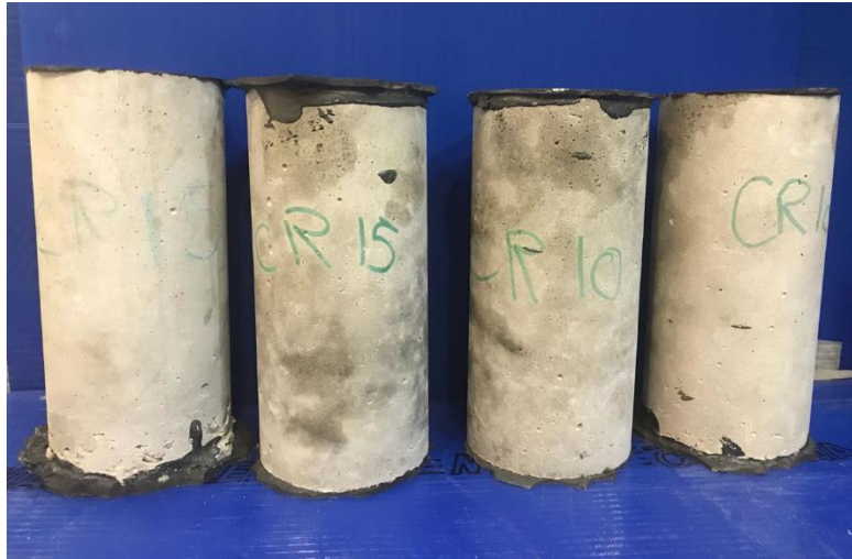
Figure 7.16 Capped cylinders before testing
