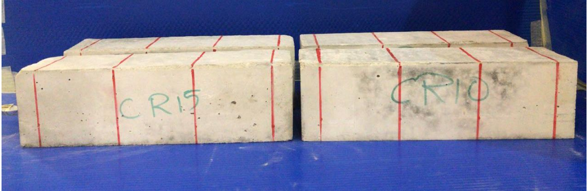
Figure 7.28 Beams (100 x 100 x 350 mm) prepared for flexural capacity test
