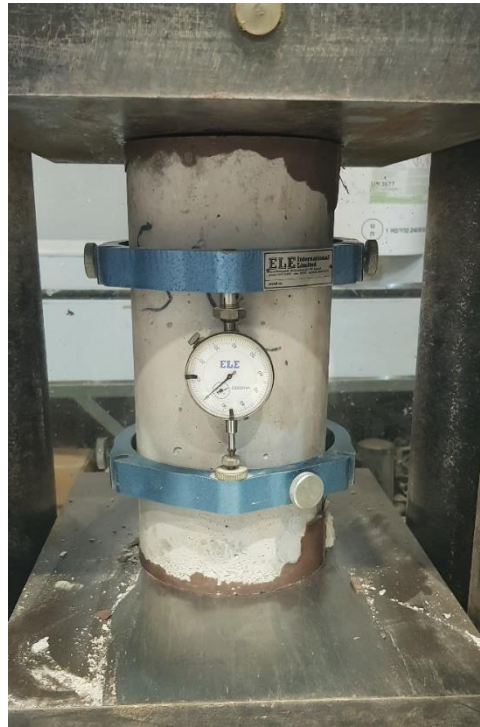
Figure 7.36 Modulus of elasticity test setup
