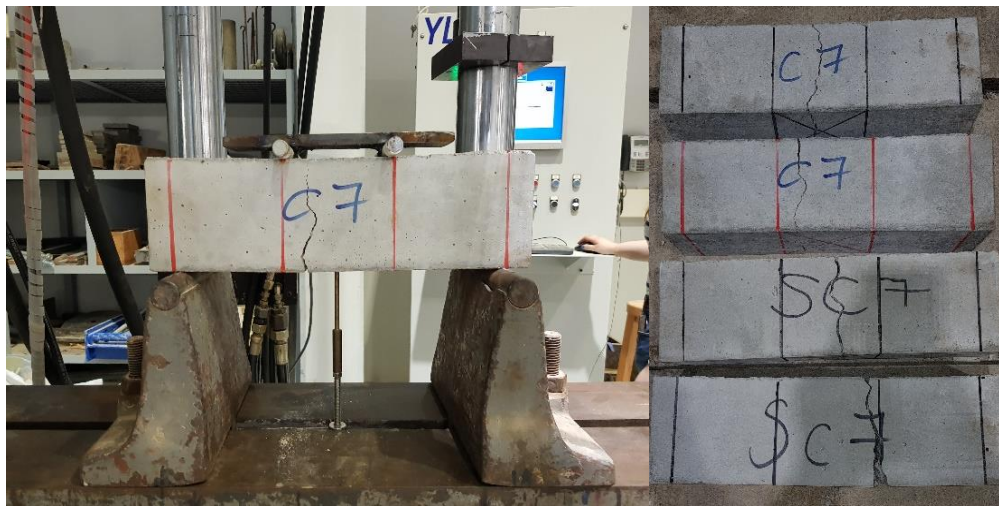
Figure 7.29 Flexural capacity test Setup
