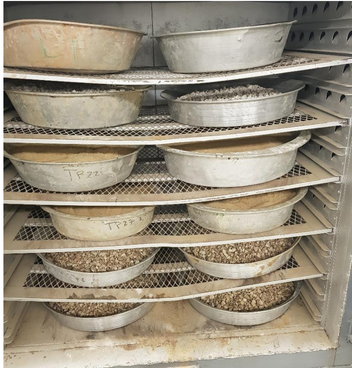
Figure 7.10 Oven dried fine and coarse aggregates
