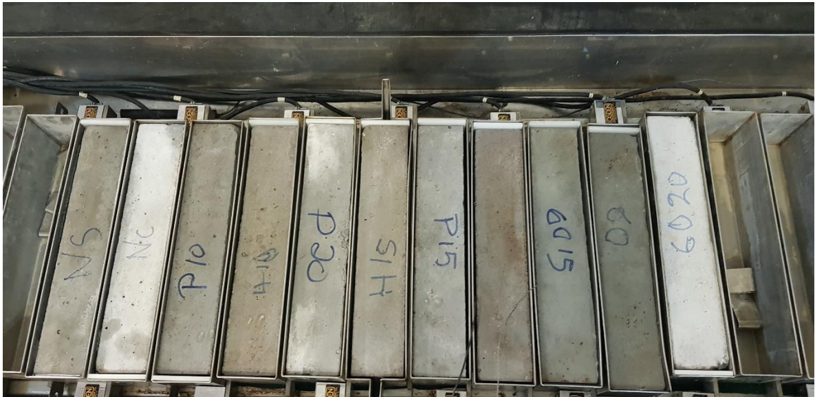
Figure 7.41 Samples inserted in the freezing and thawing machine
