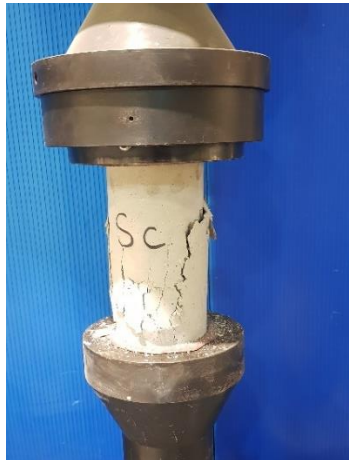
Figure 7.14 Failed Specimen after compressive strength test
