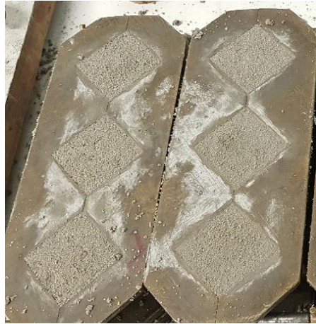
Figure 6.3 Mortar samples cast in the molds
