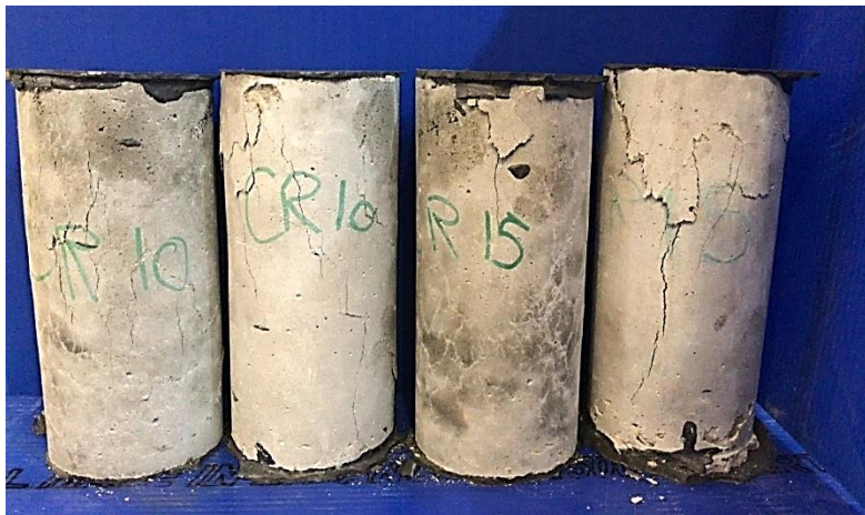
Figure 7.17 Failure modes for specimens after testing
