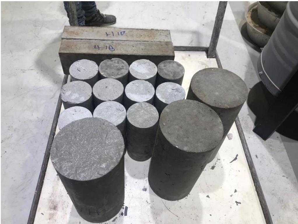
Figure 7.4 Concrete scale specimens after demolding
