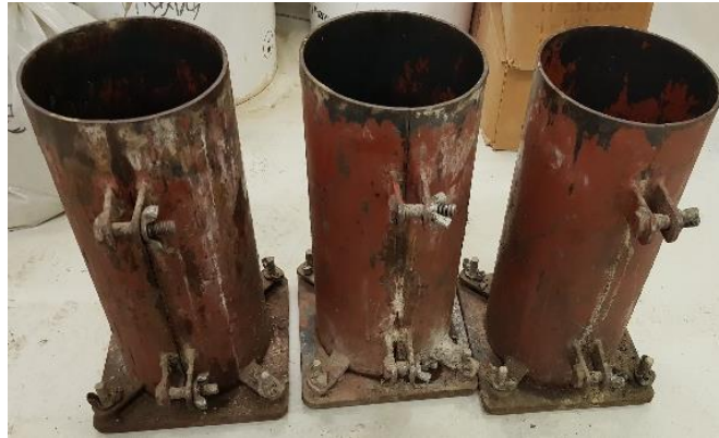
Figure 7.6 Cylindrical molds 15*30 cm
