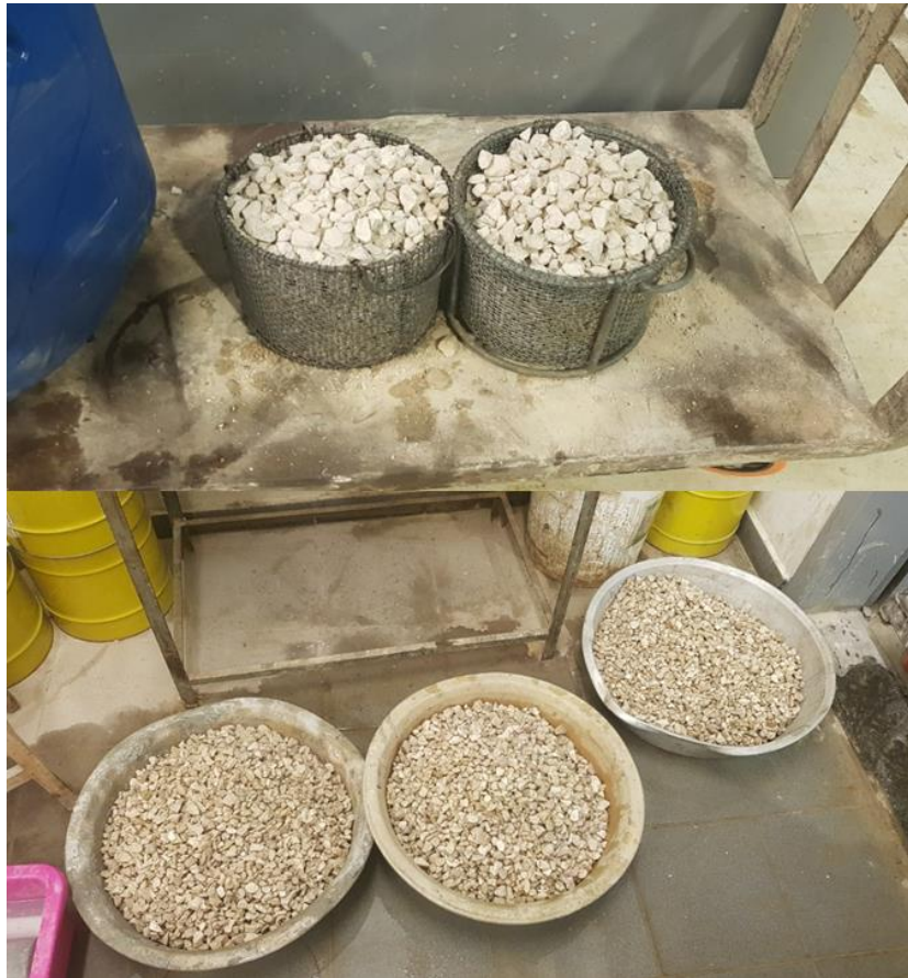
Figure 3.12 Washing coarse aggregates to remove impurities
