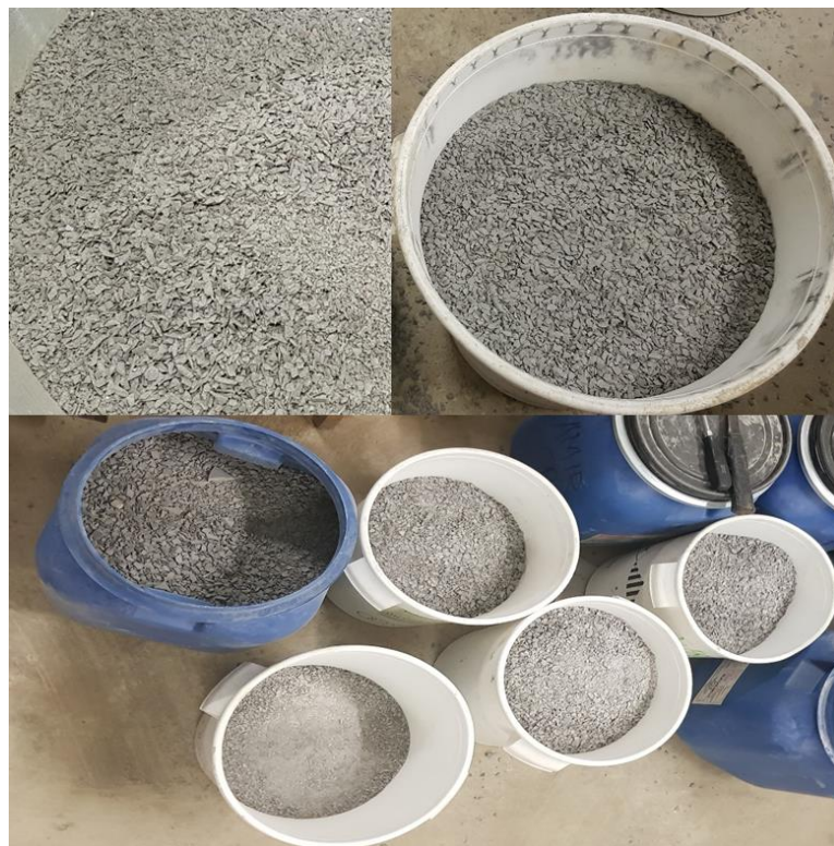
Figure 3.4 Product of the crushing machine
