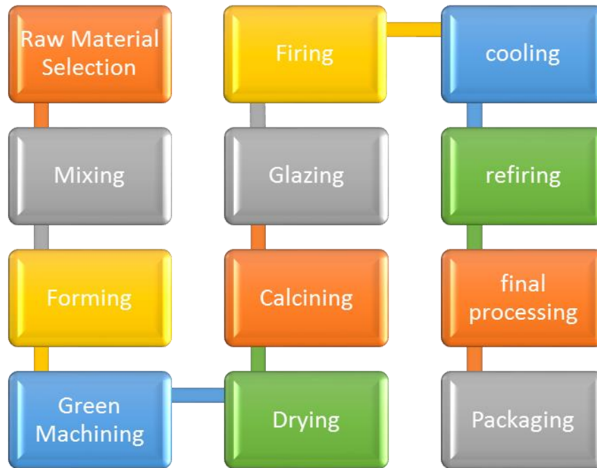
Figure 1.2 Ceramics manufacturing process
