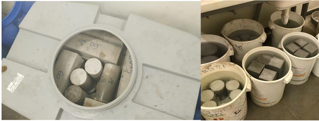
Figure 7.3 Samples cured in the water tank
