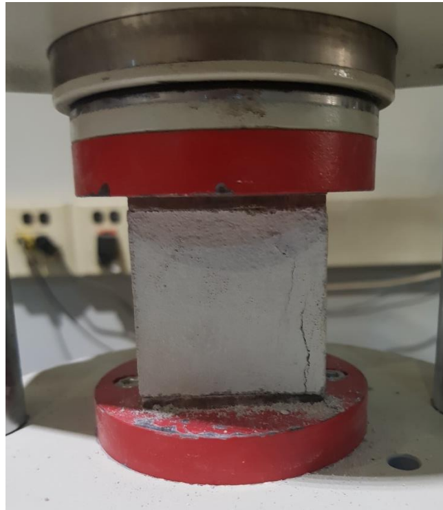
Figure 6.5 Example of a compressive strength test for mortar
