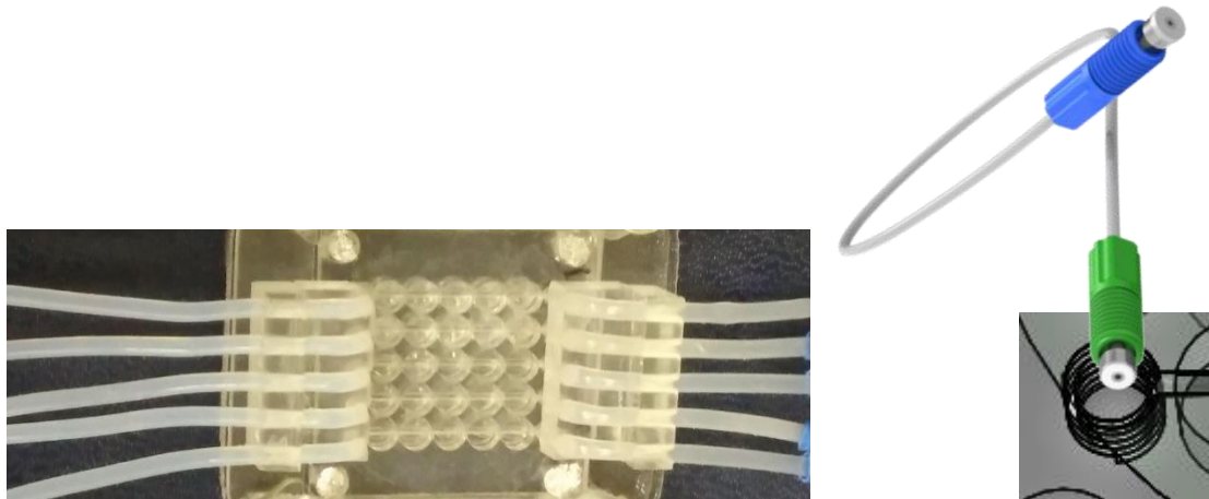
Figure 21 tube fitting and connection to LOC (a) pressure -fit tubing (b) threaded tubing PMMA chassis
