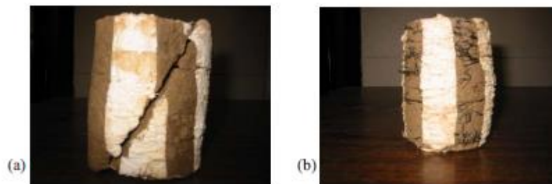
Figure 2.23 (a) Unreinforced and (b) fiber-reinforced specimen after testing (Zornberg et al., caee.utexas.edu)
