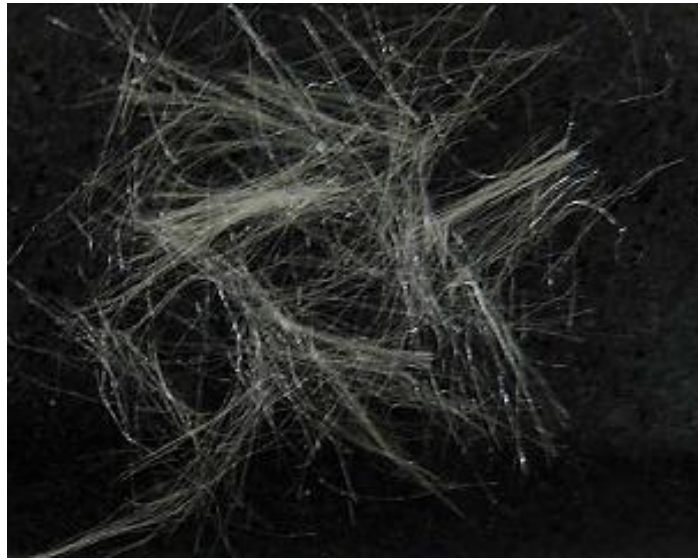
Figure 2.16 Photo of polypropylene fibers (Jiang et al., 2010)
