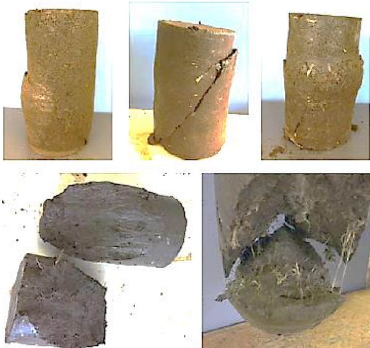
Figure 2.31 Illustration of how fibers arrest the shear plane (Najjar et al., 2014)
