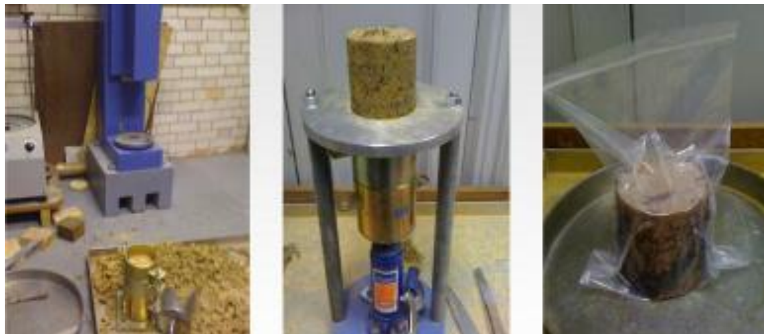
Figure 2.9 Compaction procedure (Ekinici and Ferreira (2012))
