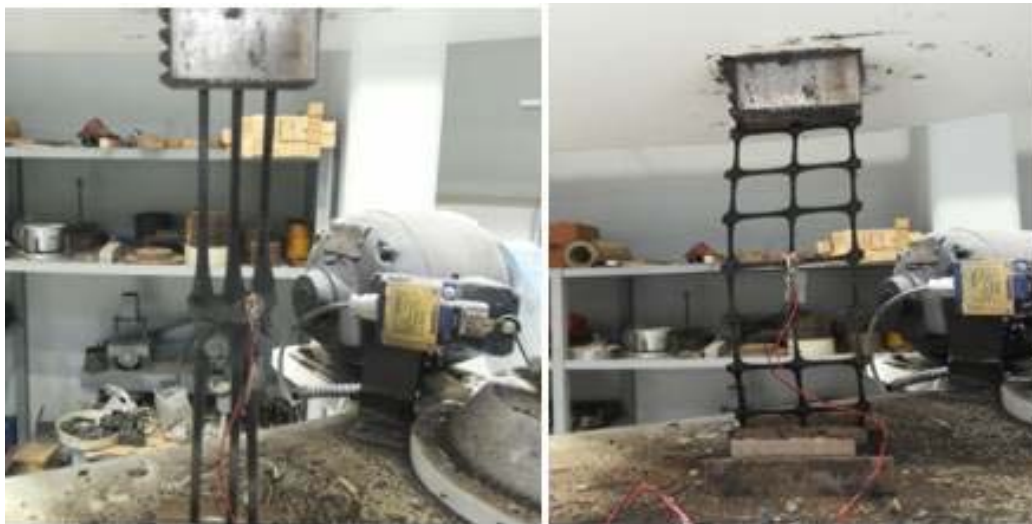
Figure 19 Direct tension test on (a) Uniaxial Geogrid (b) Biaxial Geogrid
