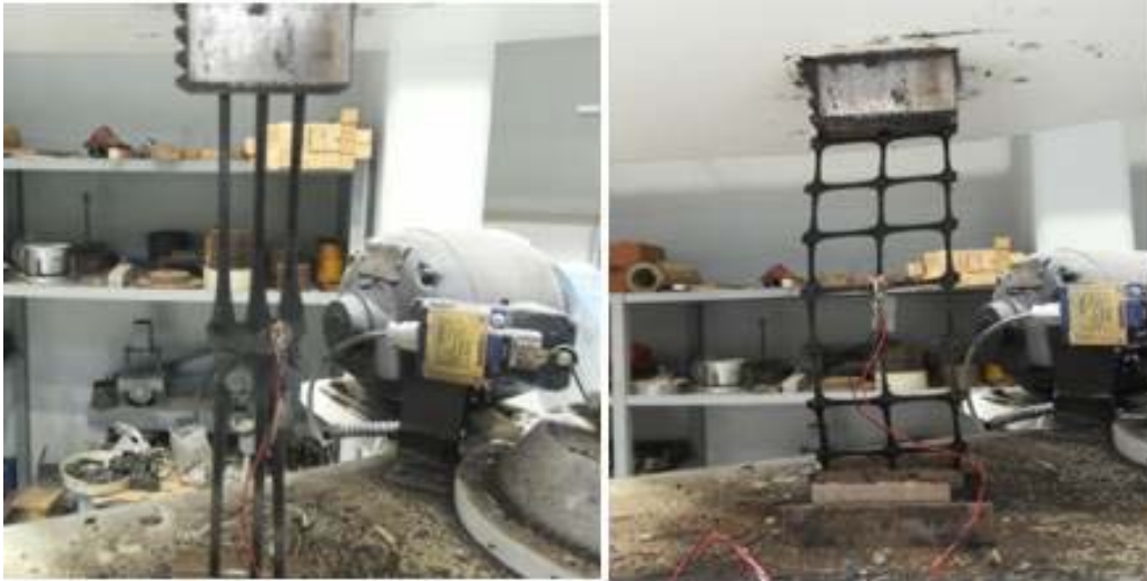
Figure 5 Direct tension test on (a) Uniaxial Geogrid (b) Biaxial Geogrid
