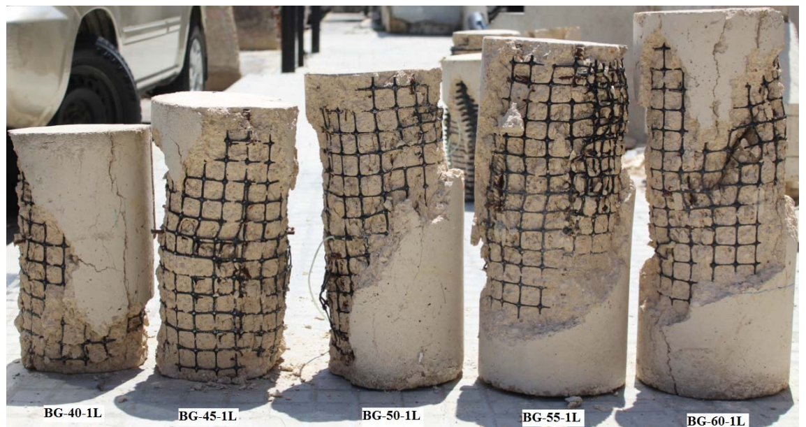
Figure 32 Failure of specimens with different slenderness ratios
