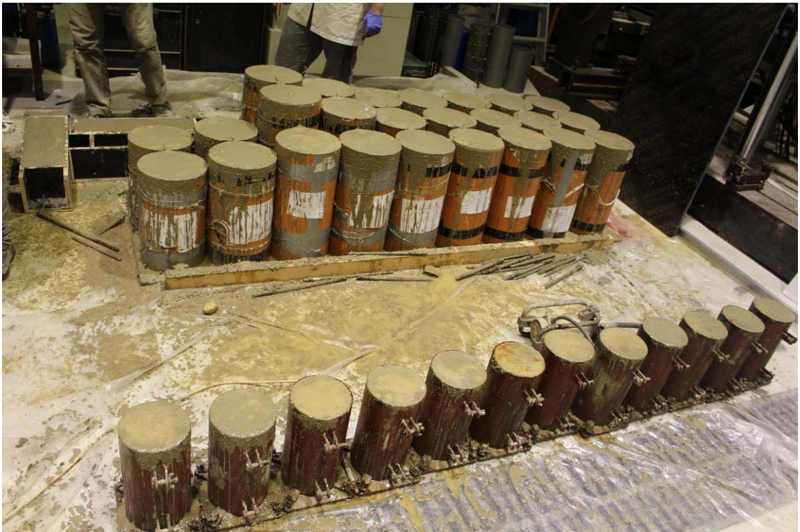
Figure 26 Casting of concrete columns
