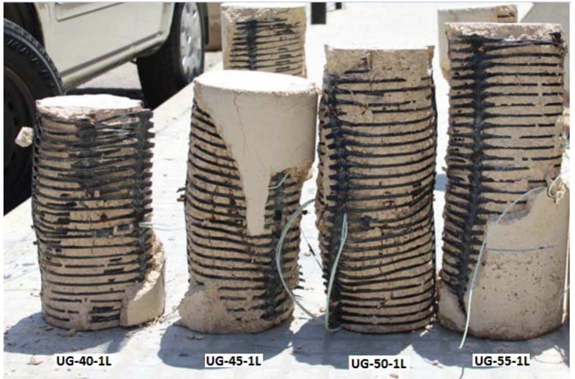
Figure 45 Failure of specimens with different slenderness ratios
