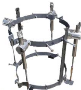
LVDT Linear Variable Trans placement Transducer (L=38 cm, D=30 cm)
