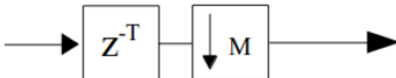
Figure A.1: T delay elements followed by an M-fold compressor
