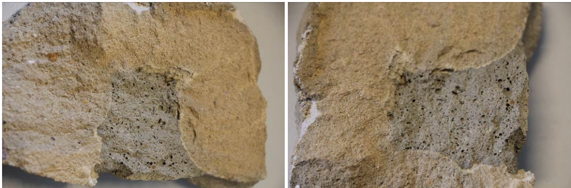
Figure 56. Difference in void sizes between extruded concrete and regularly mixed concrete
