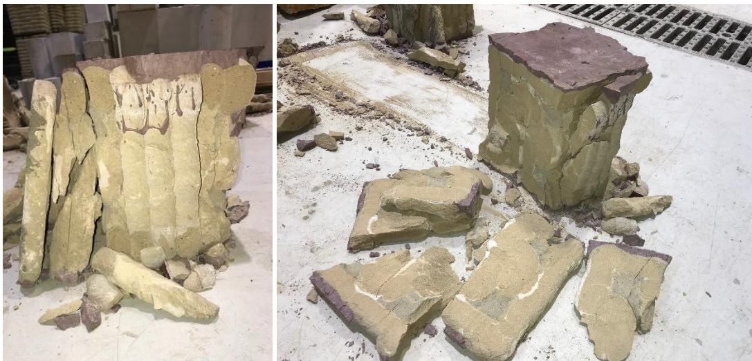
Figure 53. Concrete interlayer fracture and failure in PV:1 samples
