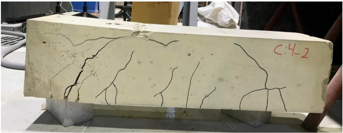
Figure 67. Cracked beam C:4-2
