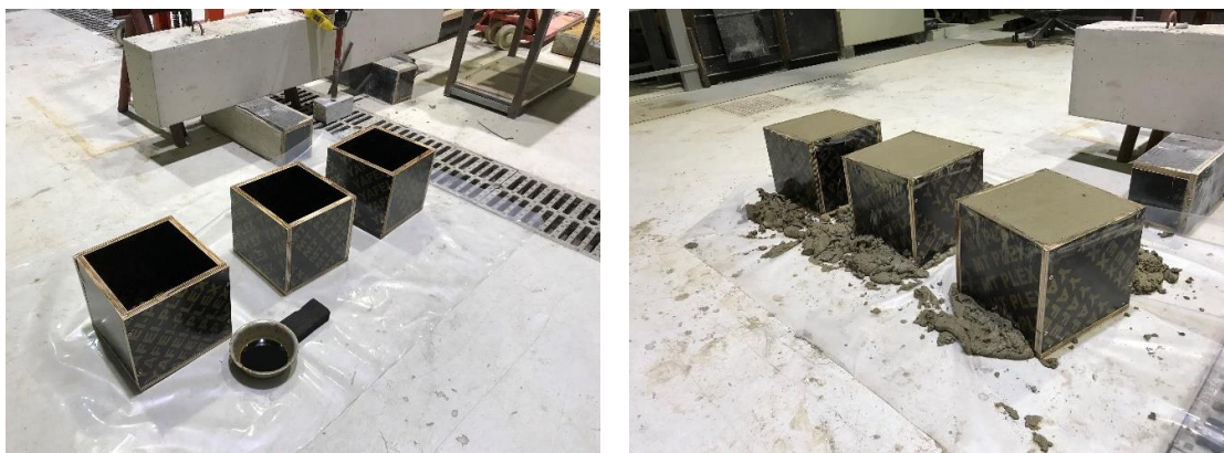
Figure 22. Molds greasing and specimens casting for C:1 samples
