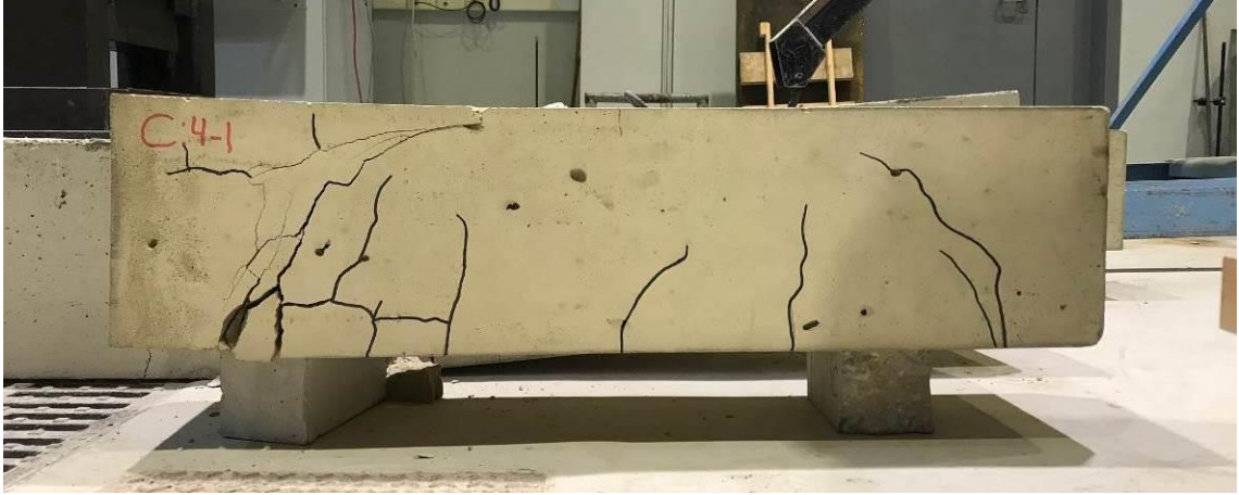
Figure 66. Cracked beam C:4-1
