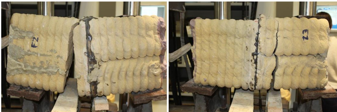
Figure 60. P:2 samples in flexure failure crack
