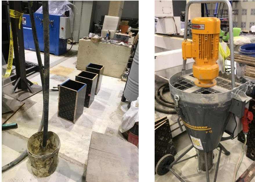
Figure 23. Mold preparation and mixer-pump used for casting C:2 specimens
