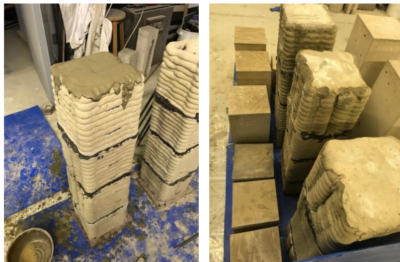
Figure 39. P:4 specimens after grouting and reinforcement insertion
