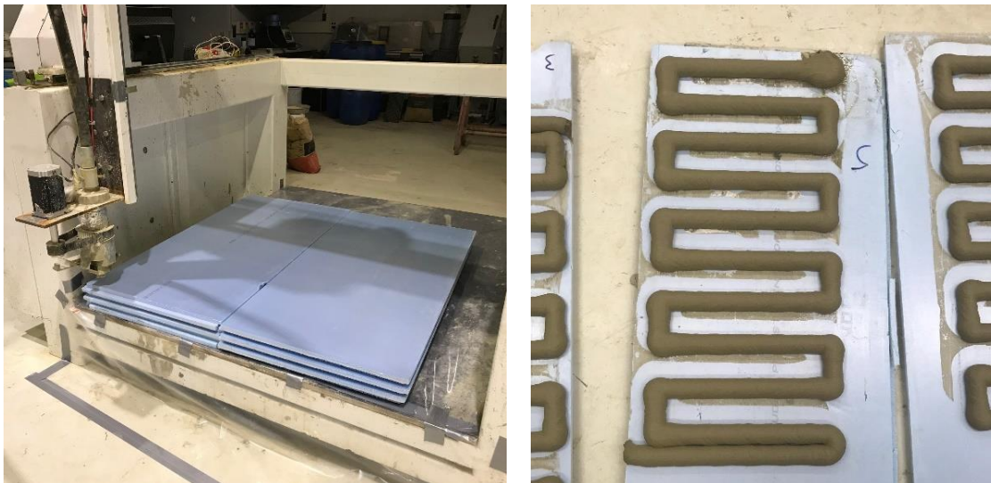
Figure 19. Layout of three layers of Styrofoam on the printing bed and printed concrete filaments
