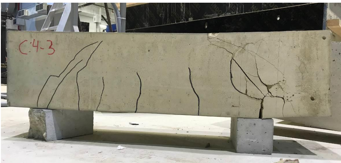
Figure 68. Cracked beam C:4-3
