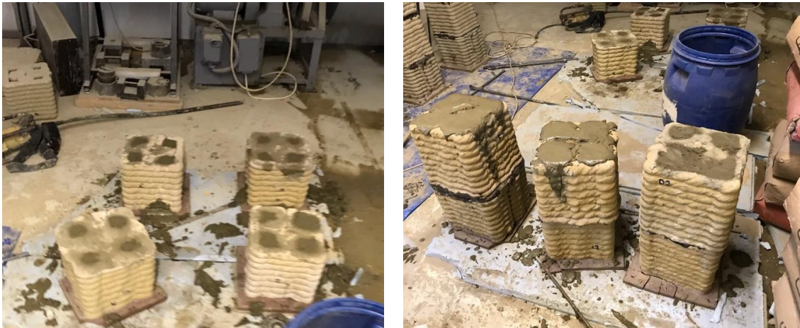
Figure 29. Samples P:1 and P:2 after grouting voids
