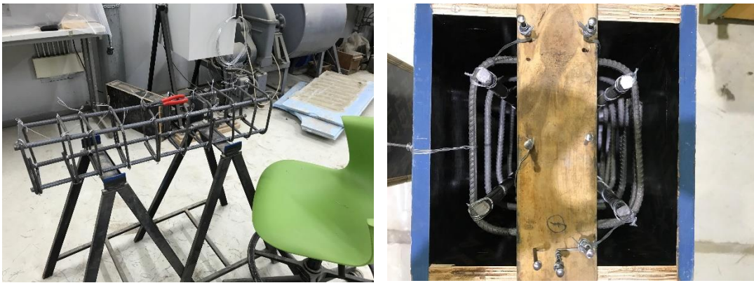
Figure 33. Steel cages preparation
