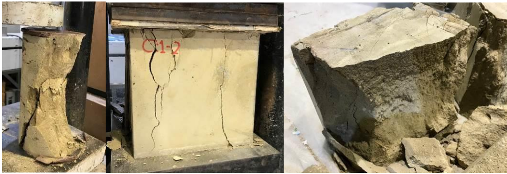
Figure 51. Cracking patterns of cast specimens
