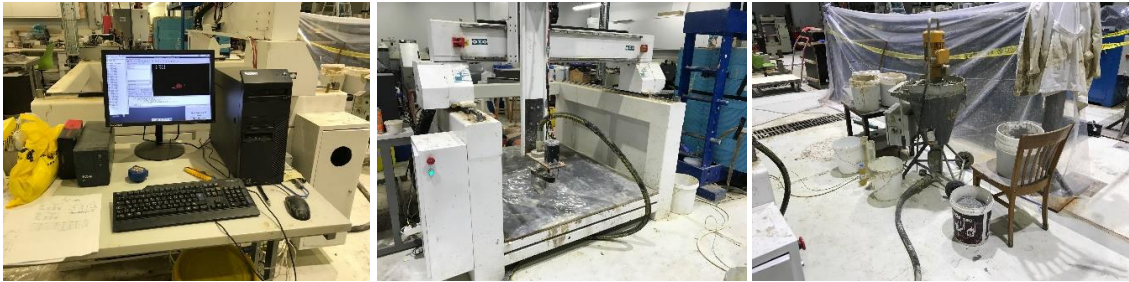
Figure 17. Components of the 3D printing system. (1) Computer hardware and software, (2) Gantry frame system, (3) Mixer-pump
