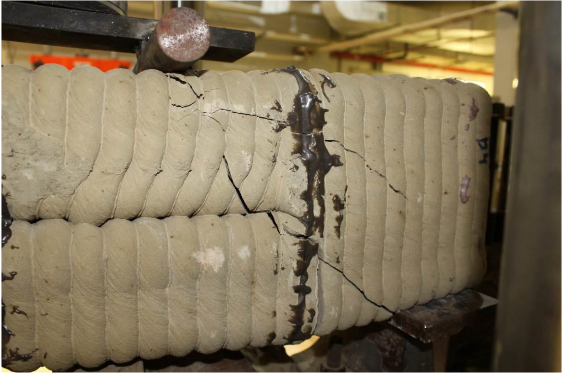
Figure 69. Cracked beam P:4-2
