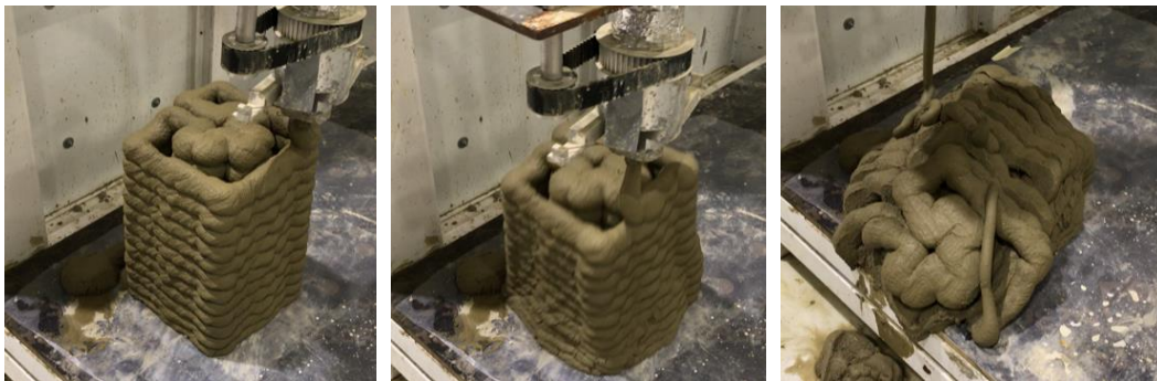
Figure 26. Failure of sample upon reaching 13 layers within a 3 minutes time-lapse.
