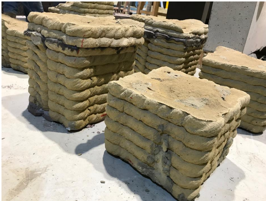
Figure 58. Interface separation in P:2 samples due to flexural failure
