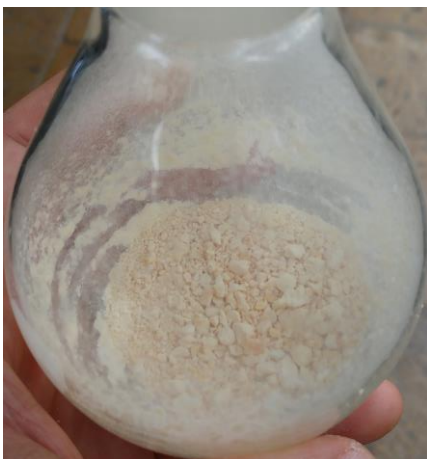
Figure 12: Final dried liposome powder of acetone washed Soy-PC.
