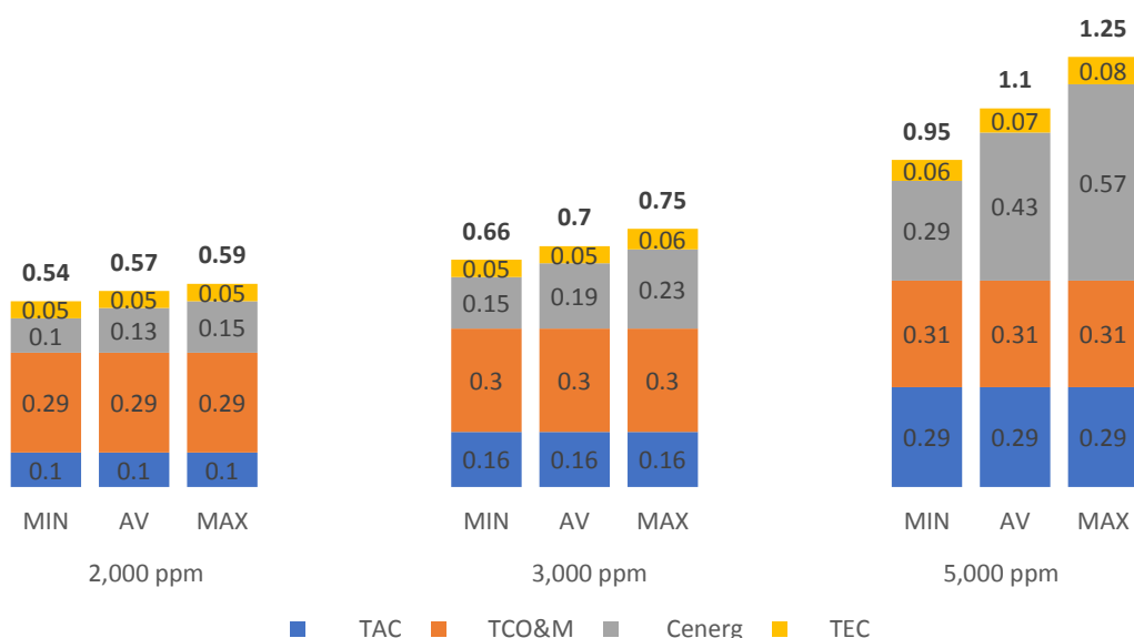
Figure 5. Cost of Desalinated Water ($/m 3 ) by Grid Powered EDR at Different Salinities Assuming an Electricity Price of 0.22 $/kWh. MIN, AV, and MAX represent the minimum, the average, and the maximum specific energy. TAC stands for the total annualized cost, TC O&M the total operation and maintenance cost, C Energ is the cost of energy, and TEC is the total environmental cost.
