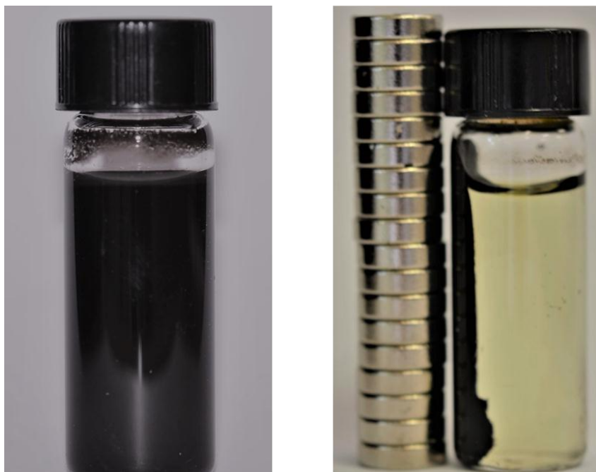
Figure 4.5: The assembly of the micro-catalytic structure was evident by the clear supernatant upon applying an external magnetic field.
