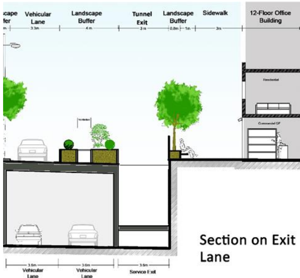
Figure 96: [“Bechara El Khoury” Tunnel Exit Section], Al Asmar 2018
