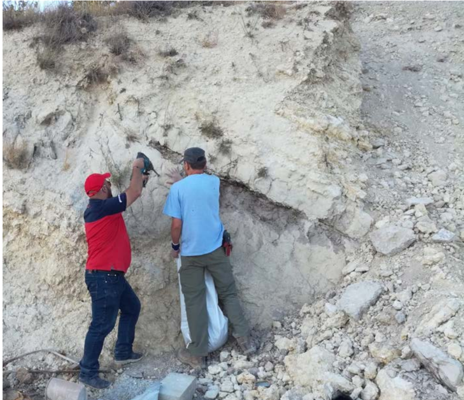
Figure 17: Picture of Drs. Fabien Knoll and George Kachacha extracting about 500 kg of sediments from sample Z-8 at section 3. Note that they are using a driller instead of a hammer to be able to extract large amount of sediments.
