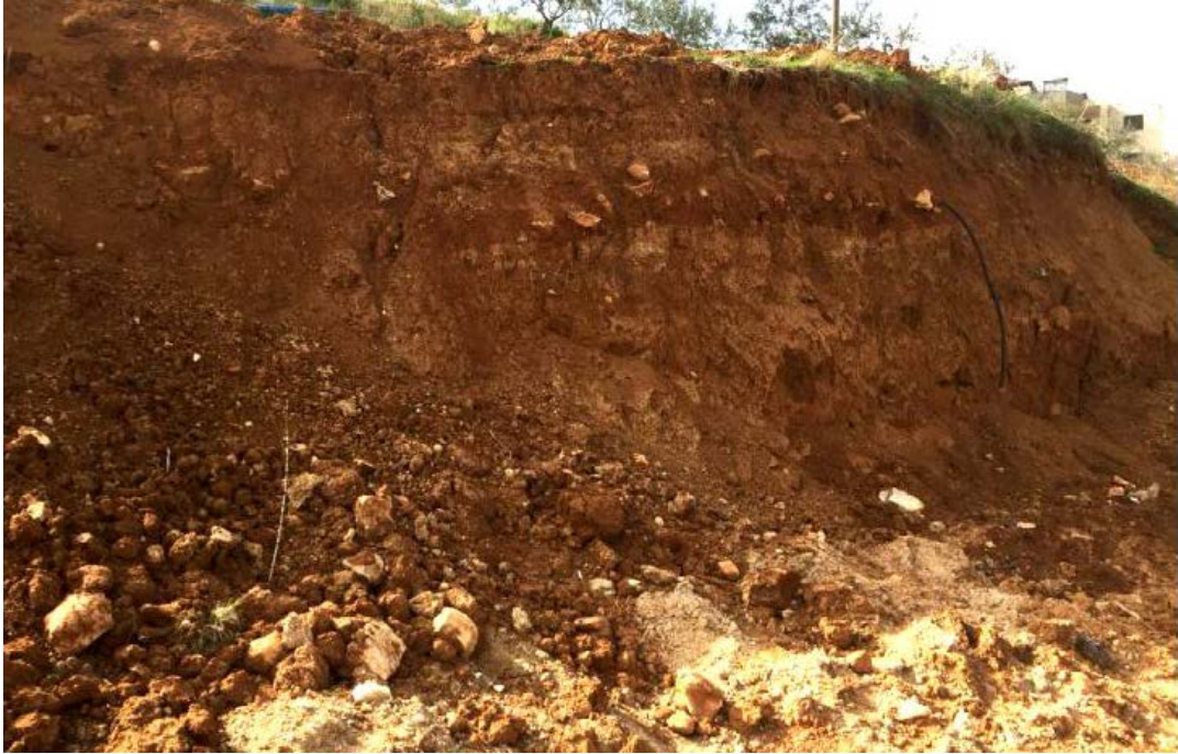
Figure 56: Field photograph of the upper part of section 6 showing the reddish clay and conglomerates.
