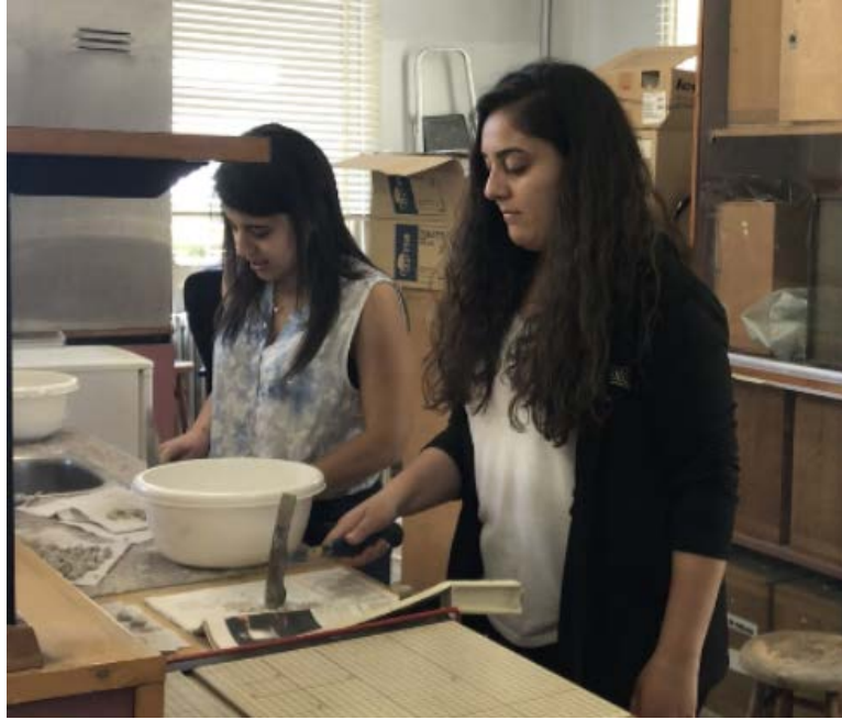
Figure 18: First stage of the sample treatment. Graduate students are removing the undesirable remains and crushing the indurated rock blocks.
