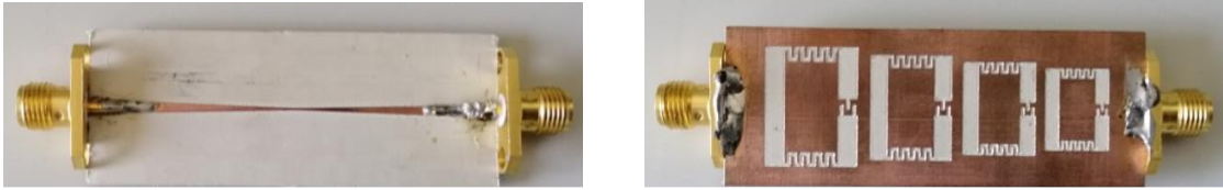
Figure 34: Top and bottom layers of a fabricated prototype of the proposed log-periodic BRF built on a 1.27 mm-thick Rogers 3006 substrate.
