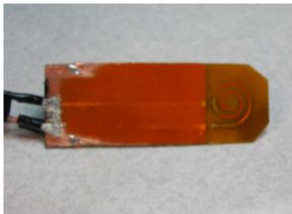
Figure 7: Spiral resonator sensor [22].
