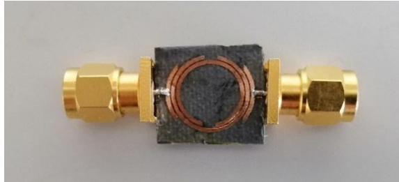
Figure 28: Fabricated prototype of the SRR-based filter.
