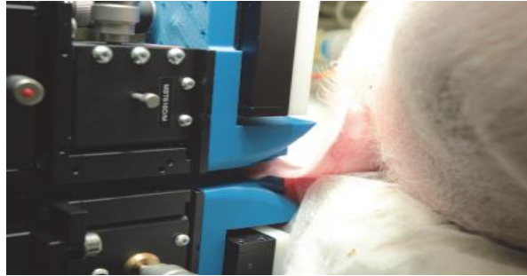
Figure 4: Tx and Rx antennas placed around pig's ear [14].
