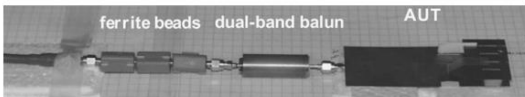
Figure 59: Ferrite beads and balun placed between the AUT and the cable for small antenna measurements [64]
