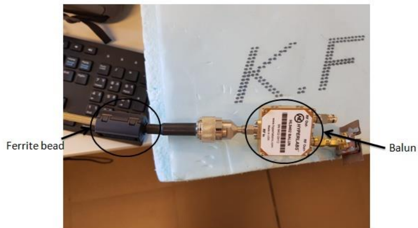
Figure 62: FMIoT antenna measurement using ferrite bead and a balun
