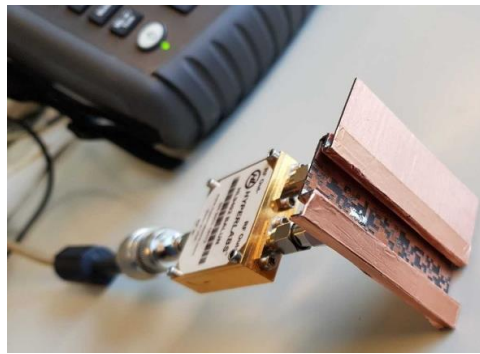
Figure 63: The prototype under measurement using a ballun and a ferrite bead
