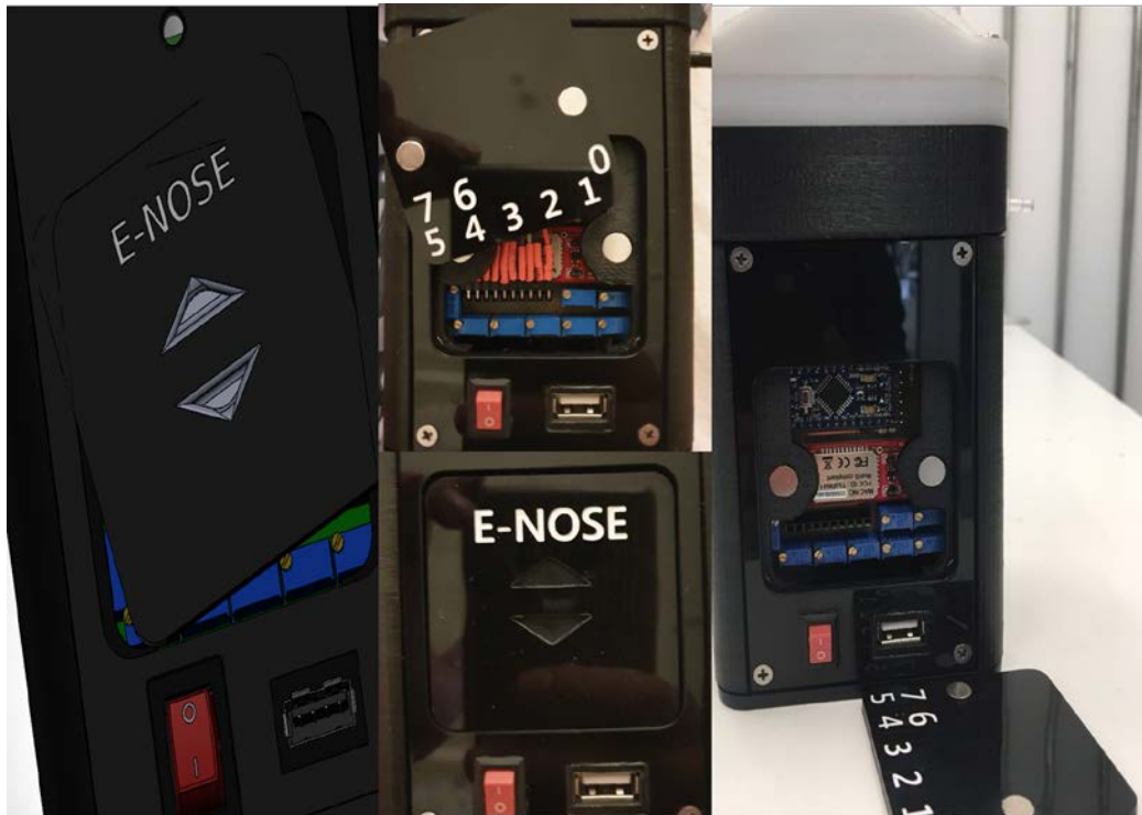
Fig. 3: A magnetic cover gives access to the variable resistors controlling the sensors
