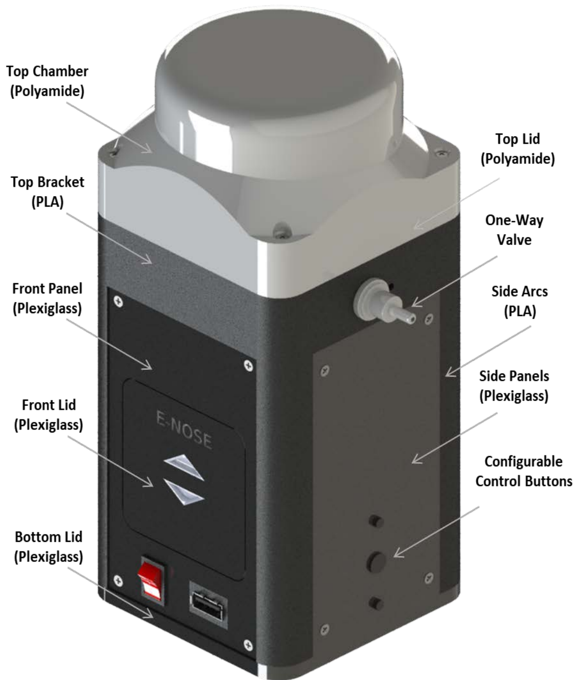
Fig. 7a: A 3D rendering of the proposed e-nose
