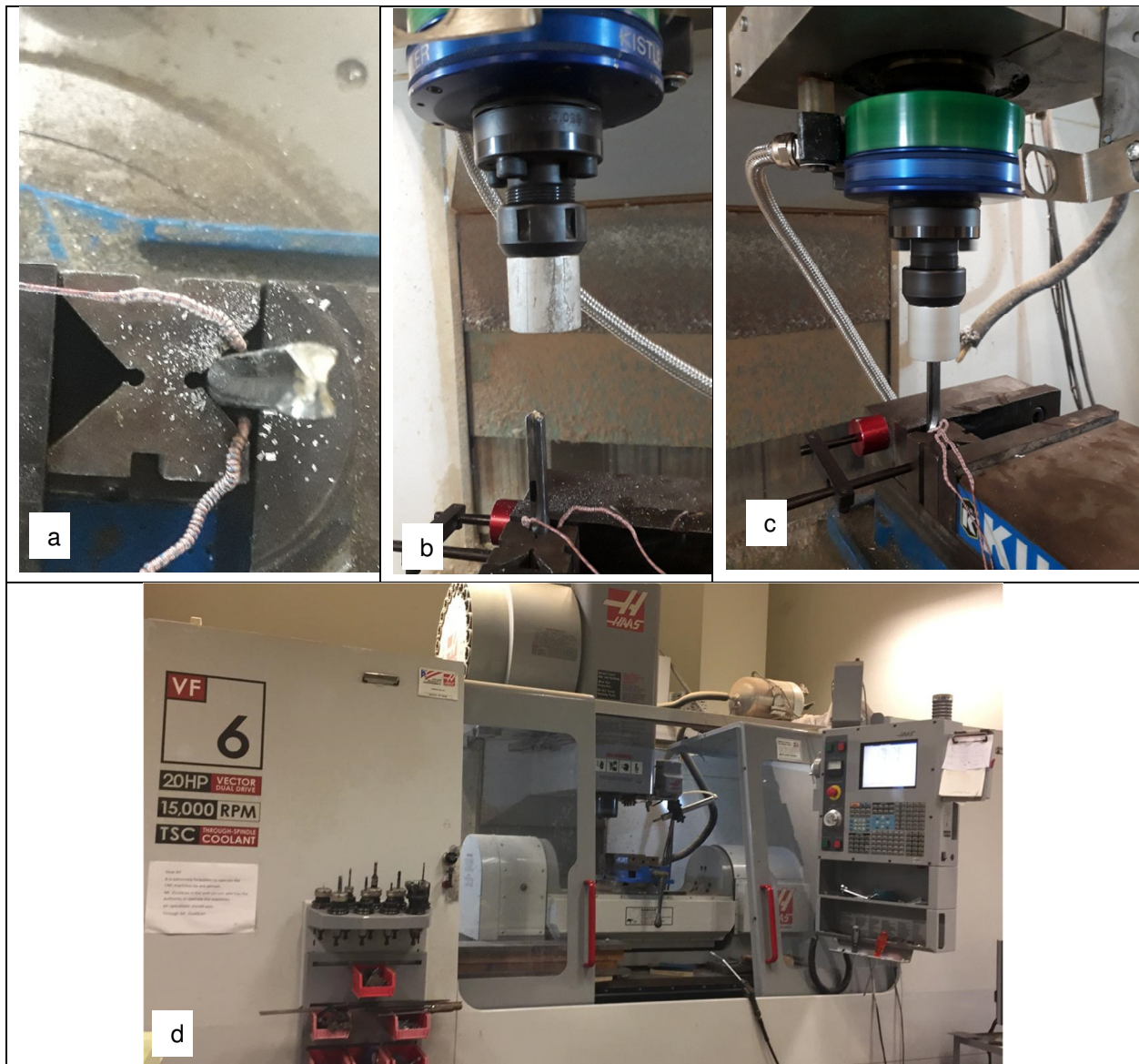
Figure 6.2 Photograph reporting a) Drill with brazed thermocouples fixed in inverted positions b) Inverted Drilling Set up c) Drilling experiment following inverted setup d) Machine Center.
