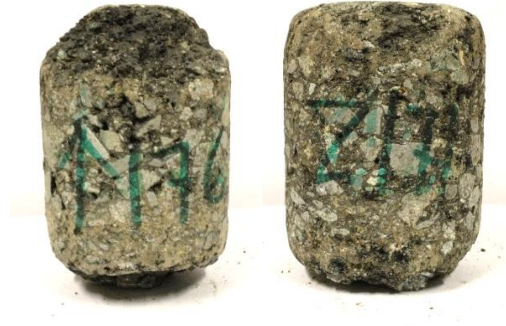
Figure 18- Asphalt samples after conducting Cantabro Test
