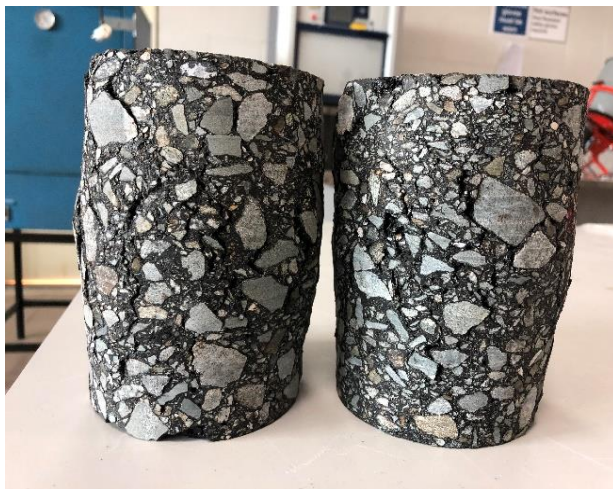
Figure 12- Damaged asphalt samples after flow number testing
