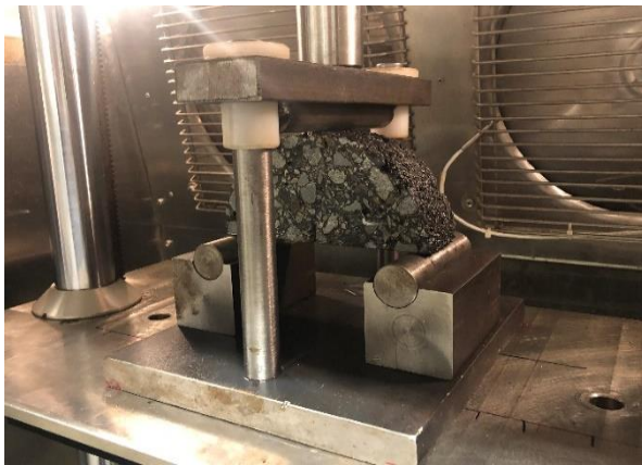
Figure 13- Semi-circular asphalt samples under SCB testing
