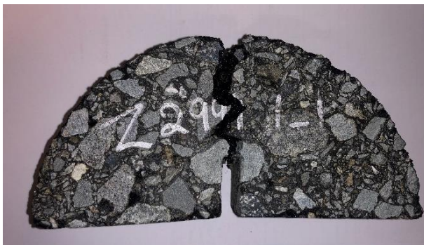
Figure 14- Damaged semi-circular asphalt samples
