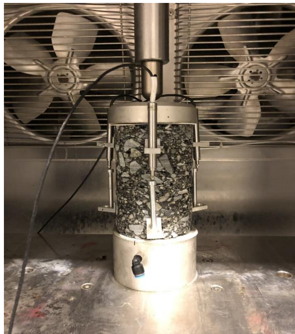
Figure 9- Asphalt sample under testing using 3 spring loaded linear variable differential transducers (LVDTs)
