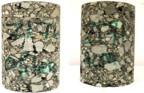
Figure 17- Asphalt samples before conducting Cantabro Test
