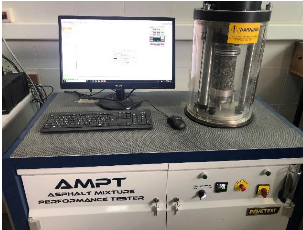
Figure 11- Asphalt sample under flow number testing
