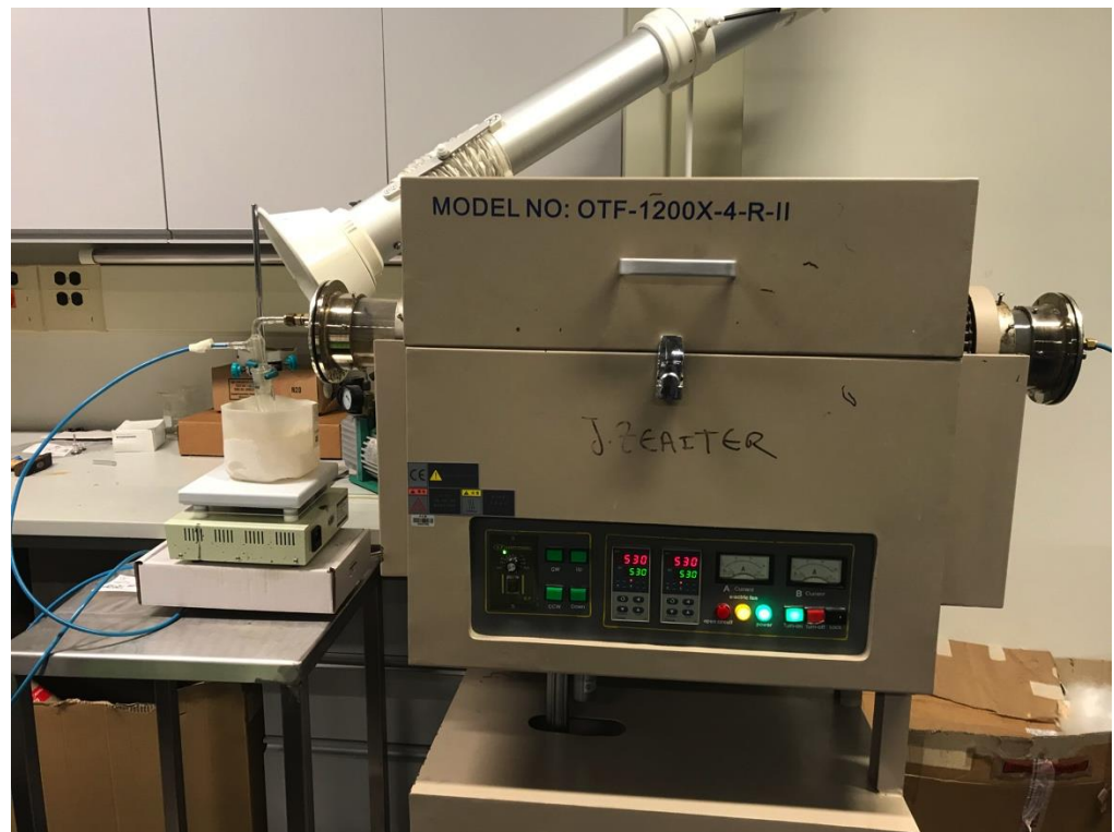
Figure 32: HDPE cracking set-up
