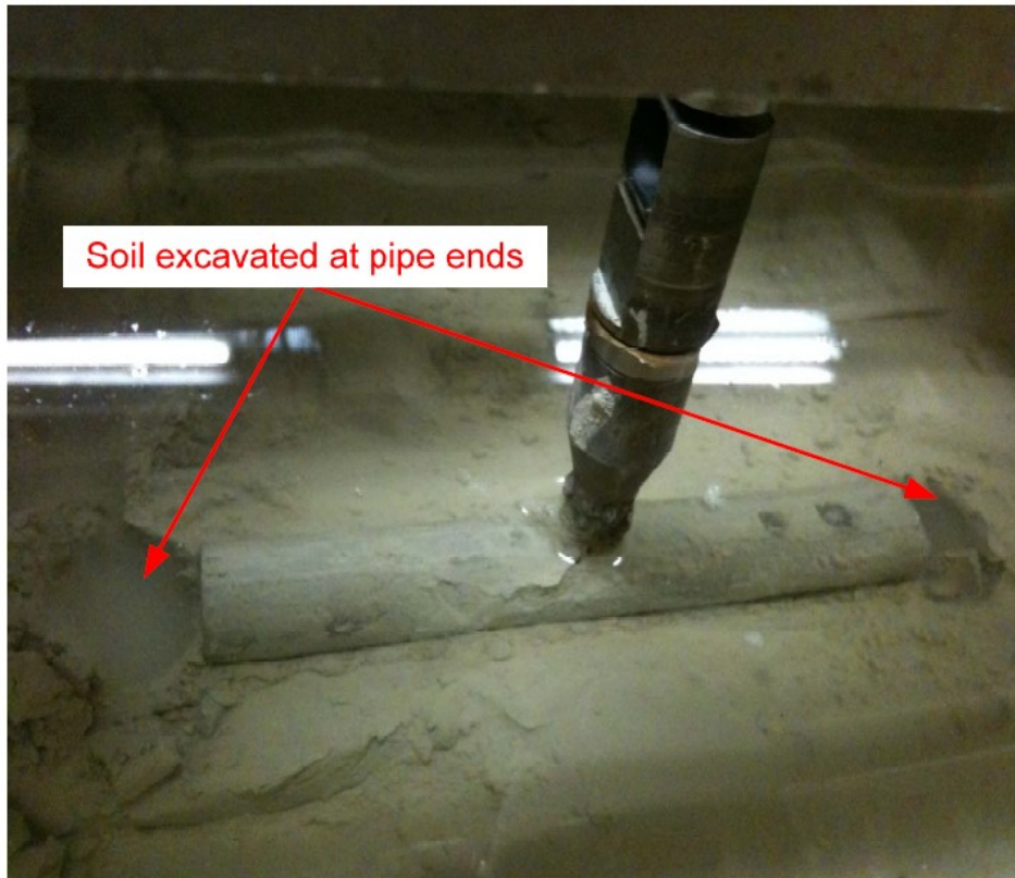
Figure 16 - Test arrangement showing clearance of soil at pipe ends.
