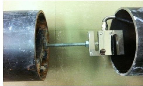
Figure 8 - Connection of load cell between the test and end sections
