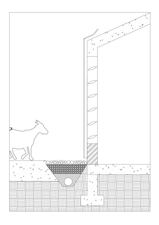
Sloped roofs used for rainwater collection are gathered by the gutter, through gravel pathway, and to rainwater reservoirs located under the concrete courtyards.
