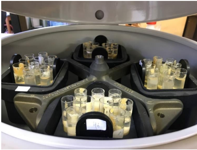
Figure 29: a) Wet samples to be separated by centrifuge device, b) Sample showing precipitated sand and gravel at the bottom, overlain by silts and clays, and water at the top.
