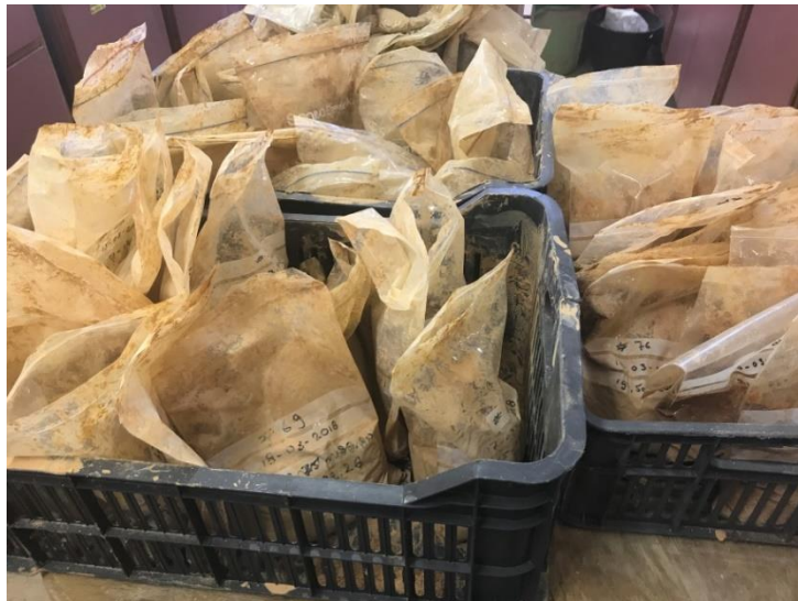
Figure 28: Cuttings samples brought to the lab from Bekaa during borehole drilling operations.
