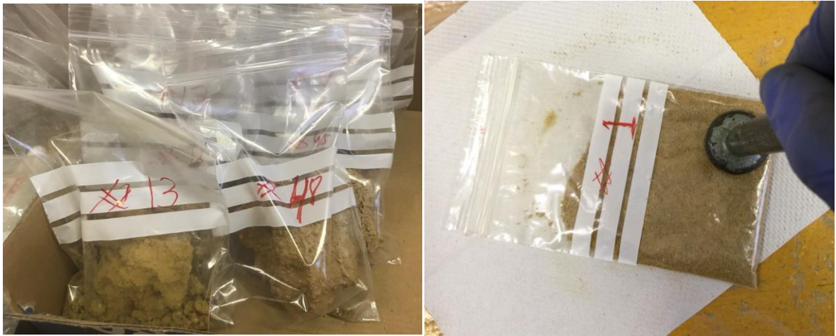
Figure 30: a) Dried samples in the oven and room temperature, b) Sample being carefully grounded by pestle.
