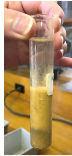
Figure 29: a) Wet samples to be separated by centrifuge device, b) Sample showing precipitated sand and gravel at the bottom, overlain by silts and clays, and water at the top.
